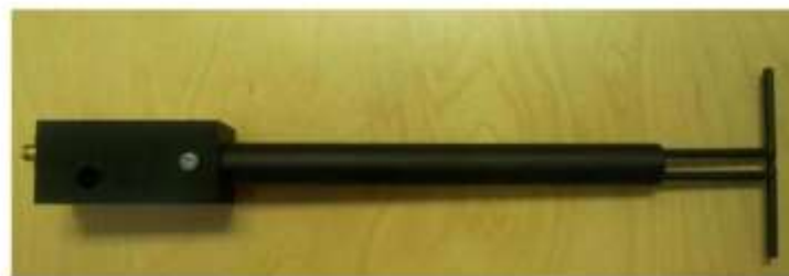
Figure 1 – MVG COMOSAR Validation Dipole
