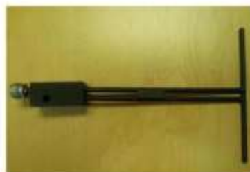
Figure 1 – MVG COMOSAR Validation Dipole
