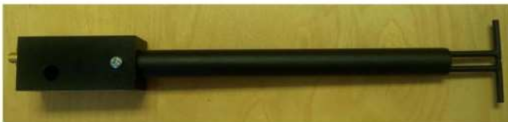
Figure 1 – MVG COMOSAR Validation Dipole
