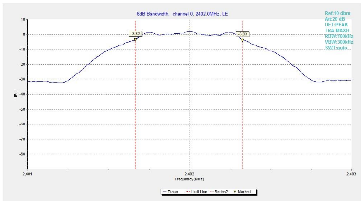
Fig.10 6dB Bandwidth (Ch 0), LE 1M
