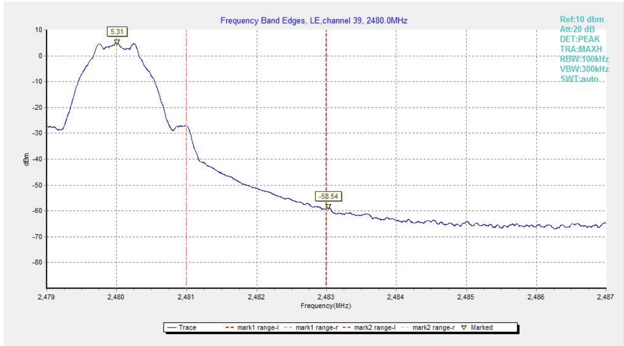
Fig.20 Band Edges (Ch 39), LE 1M
