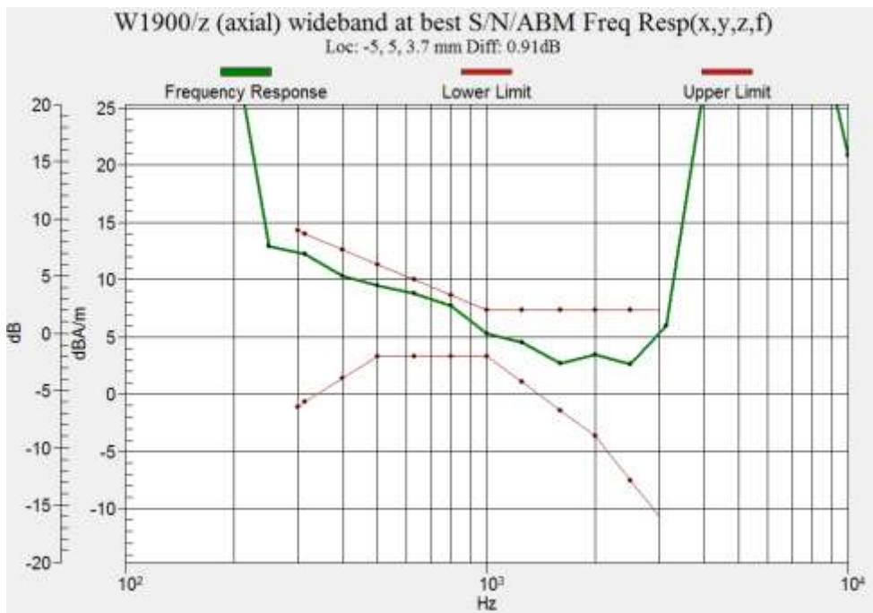
Figure B.30 Frequency Response of WCDMA Band 2 (Google Duo)
