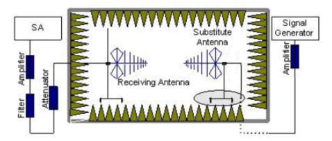
In the chamber, an substitution antenna for the frequency band of interest is placed at the reference point of the chamber. An RF Signal source for the frequency band of interest is connected to the substitution antenna with a cable that has been constructed to not interfere with the radiation pattern of the antenna. A power  $(P_{Mea})$  is applied to the input of the
