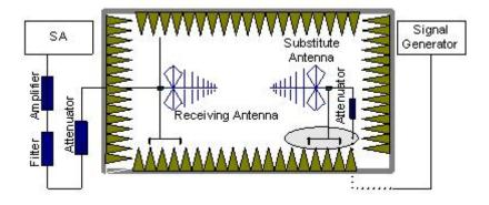
In the chamber, an substitution antenna for the frequency band of interest is placed at the reference point of the chamber. An RF Signal source for the frequency band of interest is
