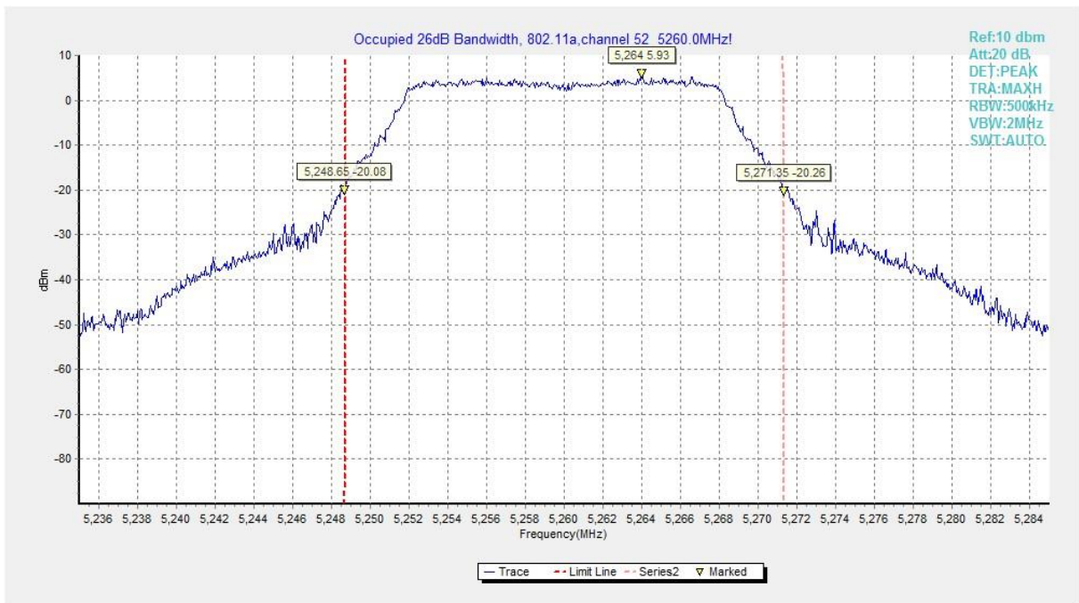
Fig. 4 Occupied 26dB Bandwidth (802.11a, 5260MHz)
