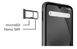
Note: Please always use the SIM ejection pin to eject the SIM card to ensure the device is not damaged.
