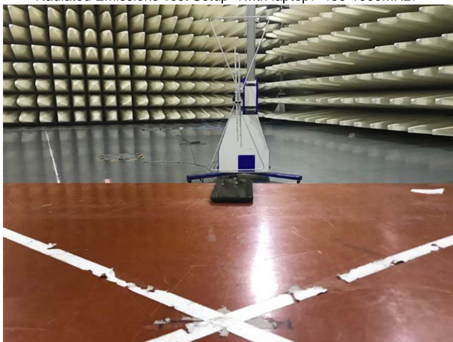
Radiated Emissions Test Setup (with charger) (30-1000MHz)
