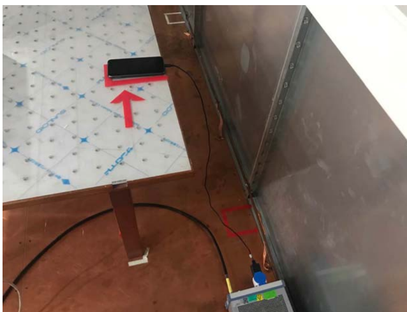
Conducted Emissions Test Setup (with charger)
