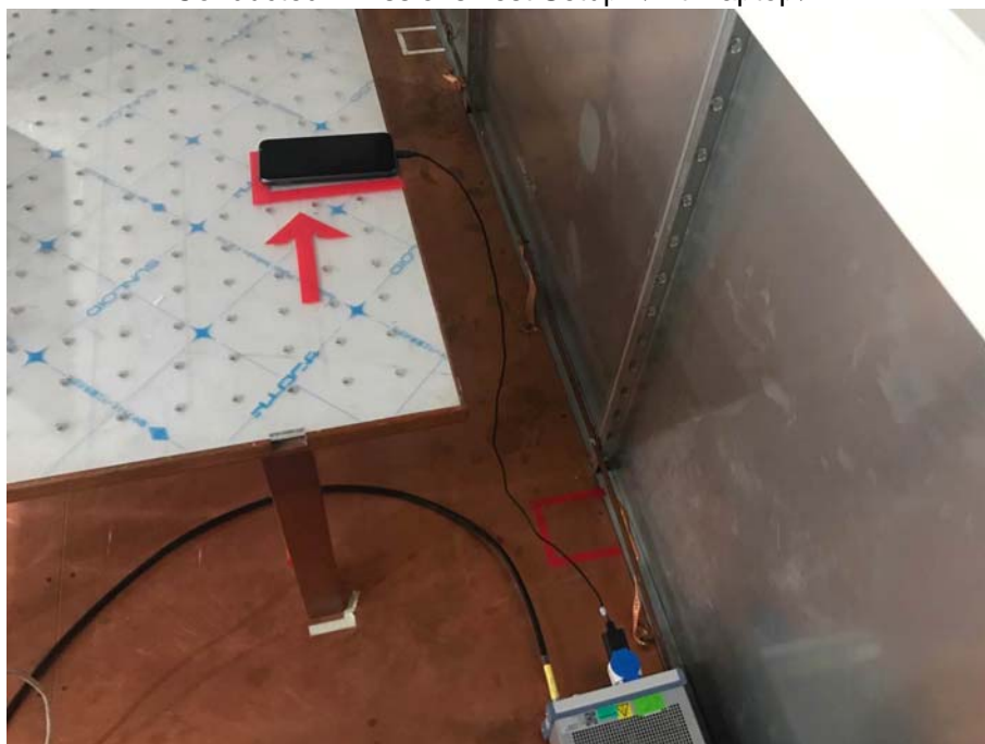
Conducted Emissions Test Setup (with charger)
