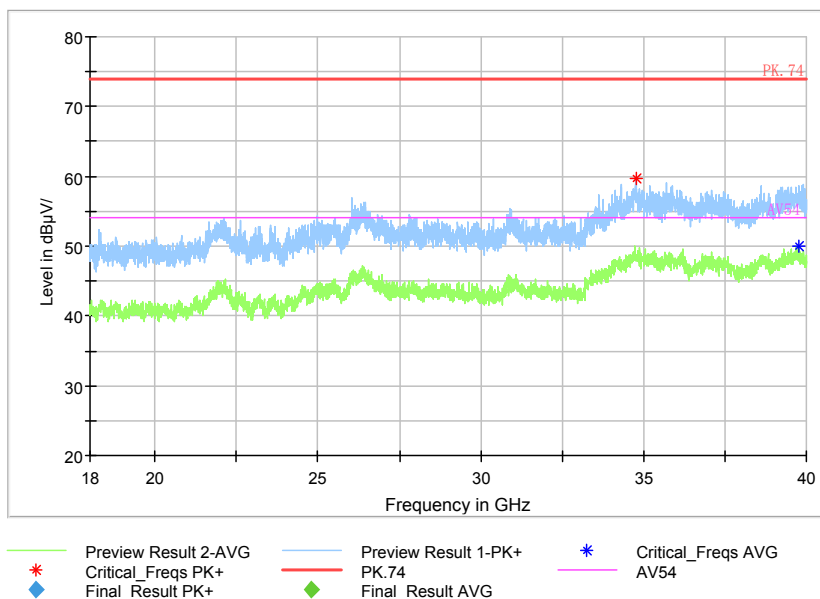
Pic12. Radiated emission (18GHz – 40GHz)
