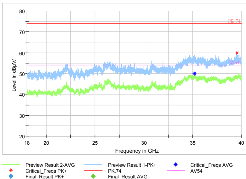
Pic8. Radiated emission (18GHz – 40GHz)
