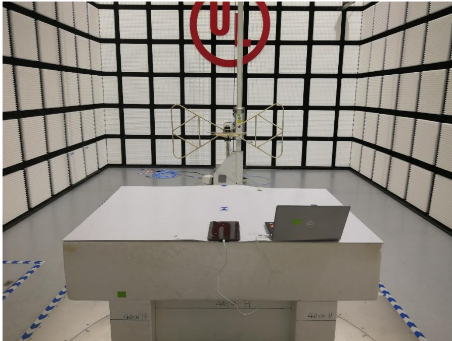
RADIATED RF MEASUREMENT SETUP (30MHz~1GHz)
