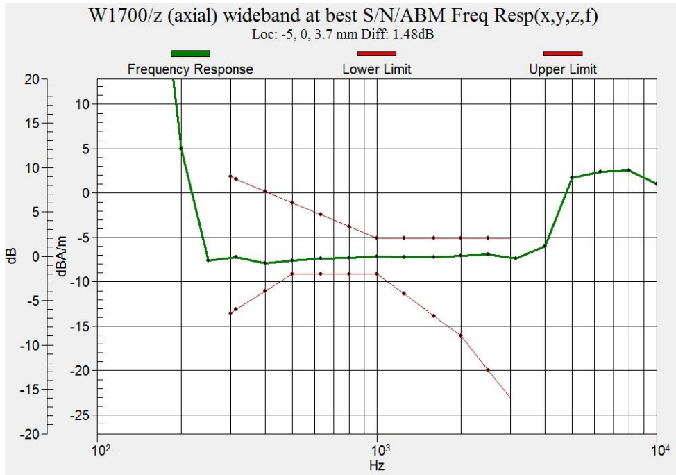
Figure B.7 Frequency Response of WCDMA B4
