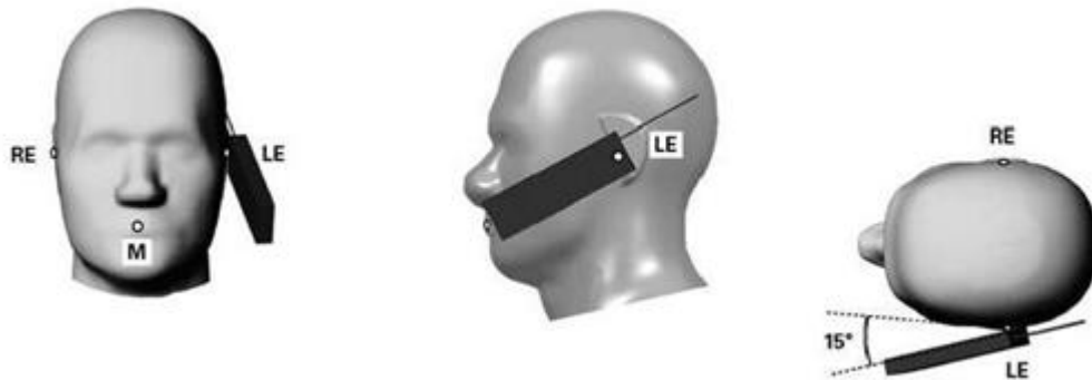
Picture17 Tilt position. The reference points for the right ear (RE), left ear (LE), and mouth (M), which define the Reference Plane for handset positioning, are indicated.
