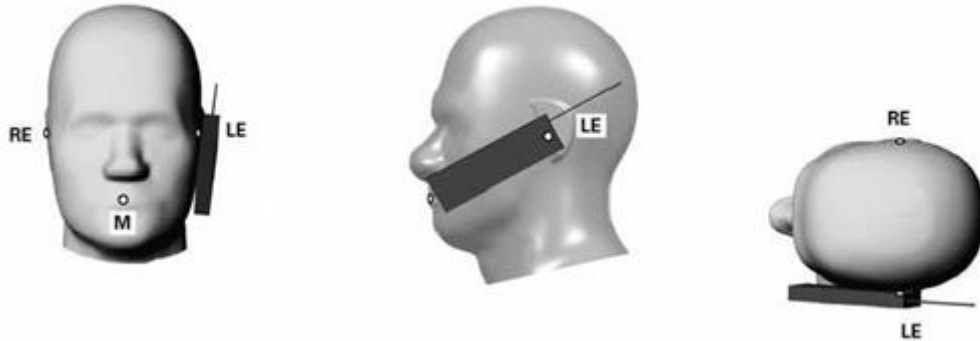
Picture16 cheek or touch position. The reference points for the right ear (RE), left ear (LE), and mouth (M), which establish the Reference Plane for handset positioning, are indicated.
