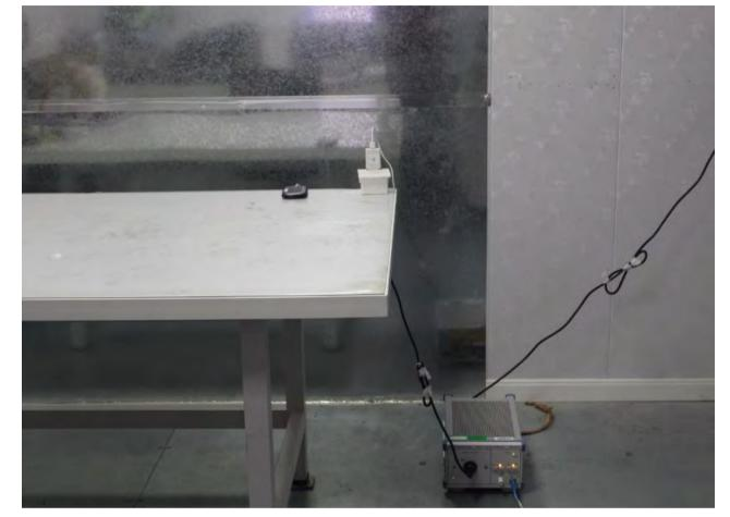
1.4 Conducted Emissions at Mains Terminals (150kHz-30MHz) Test Setup
