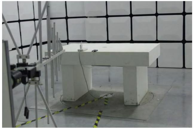
1.5 Radiated Emissions Test Setup
