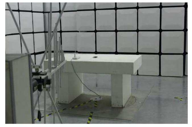
**1.6** Radiated Spurious Emissions Test setup
