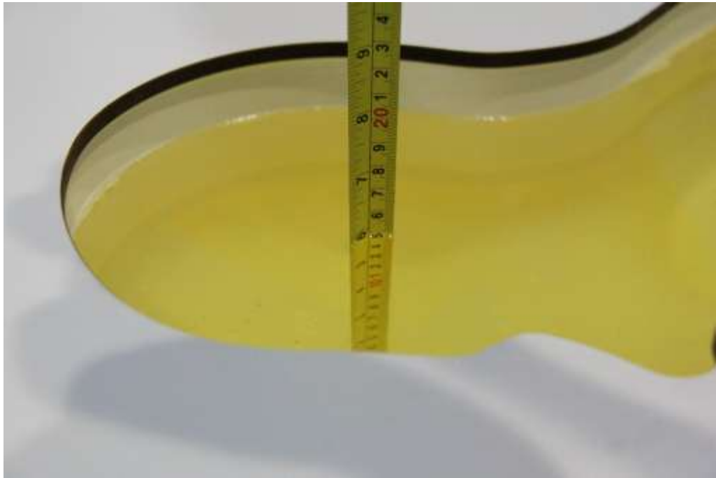
Picture 7-5: Liquid depth in the Head Phantom(2450MHz)
