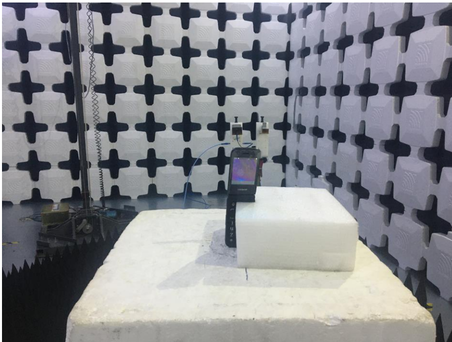
14. Radiated Emissions (Part 22/24/27/90, 18GHz -26.5GHz)
