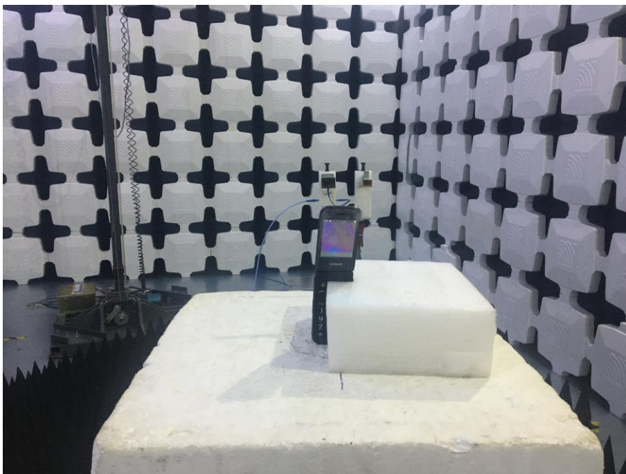
12. Radiated Emissions (Part 15C, 18GHz -26.5GHz)
