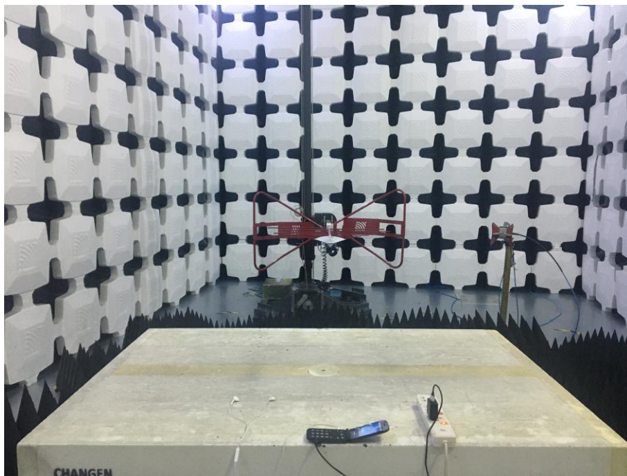
8. Radiated Emissions (Part 15B, FM receiver,1GHz-18GHz)
