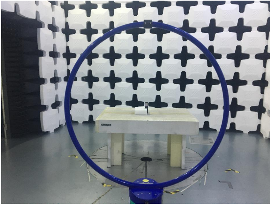
9. Radiated Emissions (Part 15C, 9kHz-30MHz)
