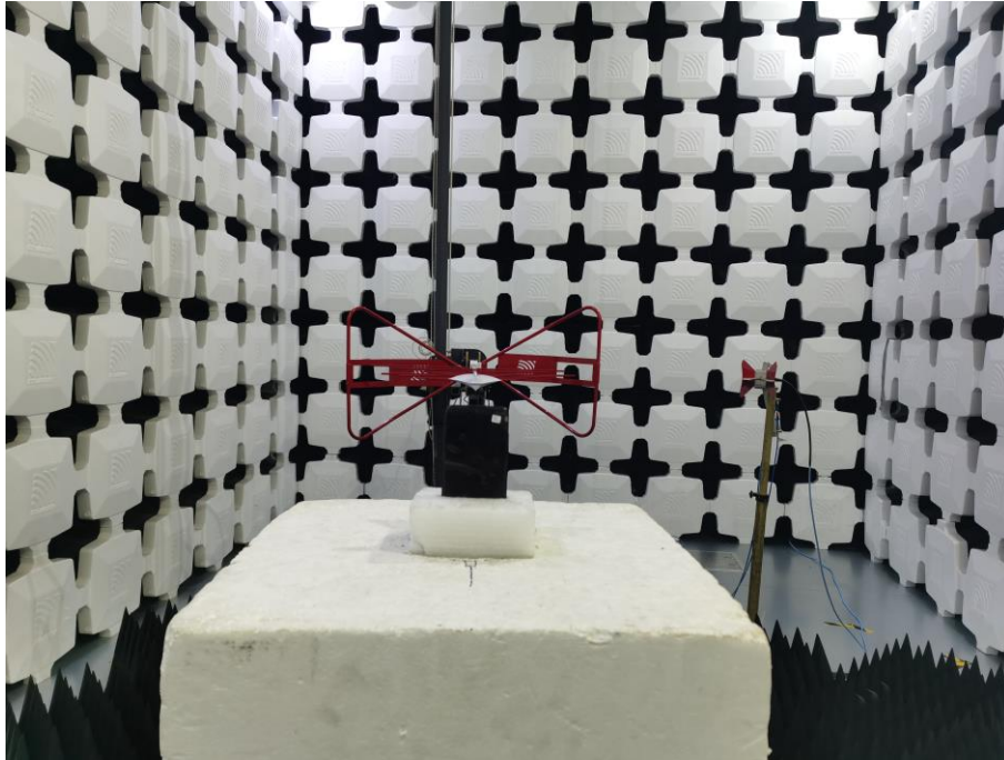
11. Radiated Emissions (Part 15C, 1GHz -18GHz)
