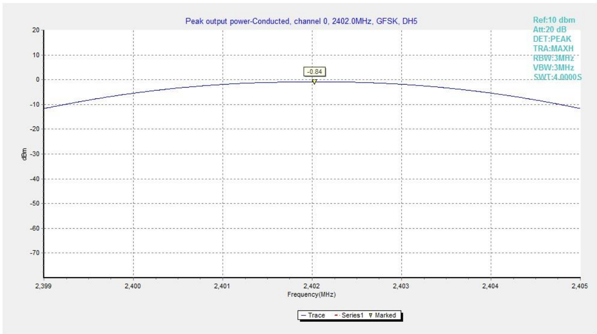
Fig. 1 RF output power (GFSK, Ch 0)
