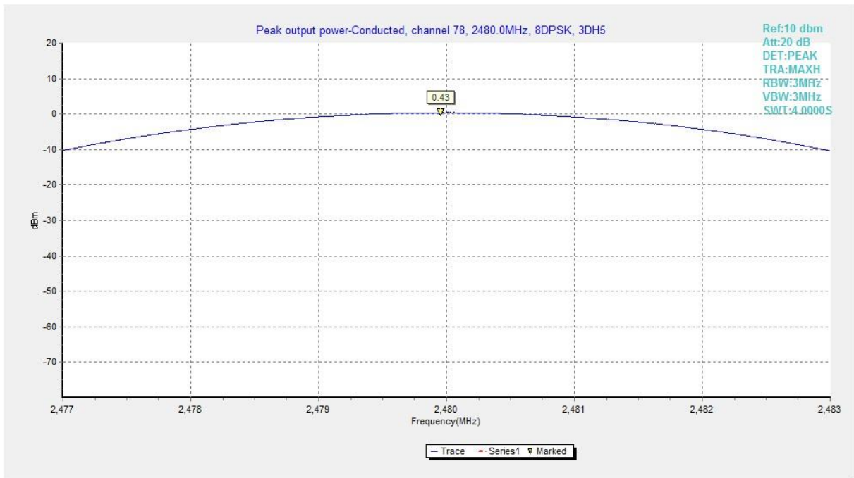
Fig. 9 RF output power (8DPSK, Ch 78)
