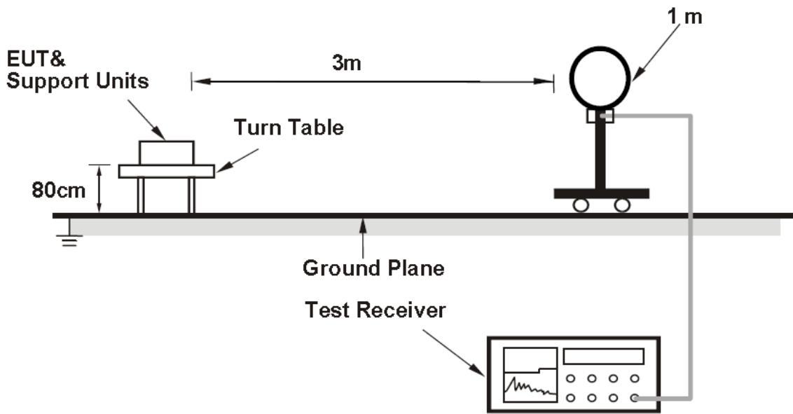
For Radiated emission 30MHz to 1GHz
