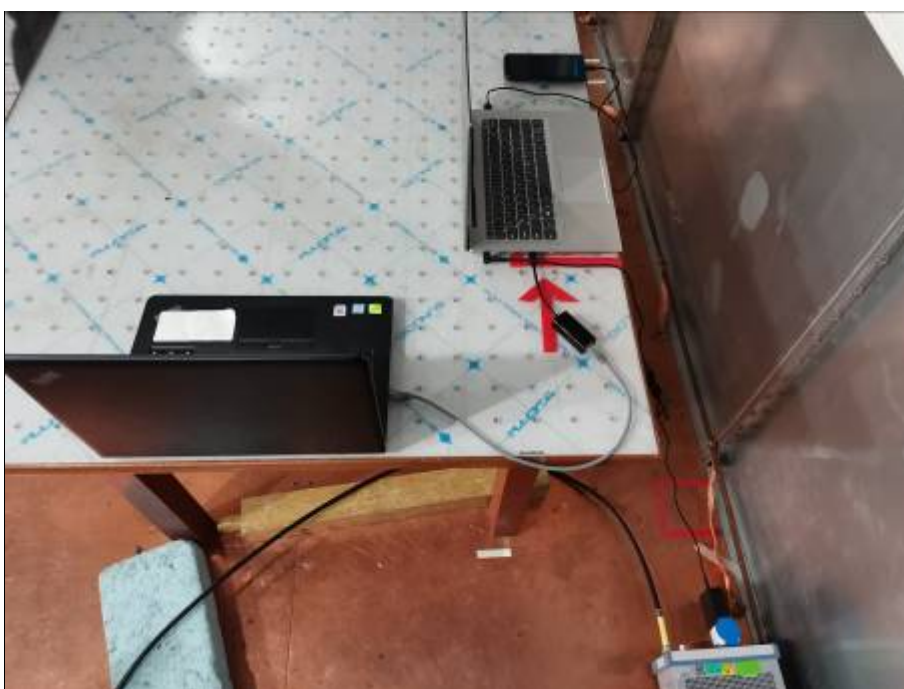
Conducted Emissions Test Setup
