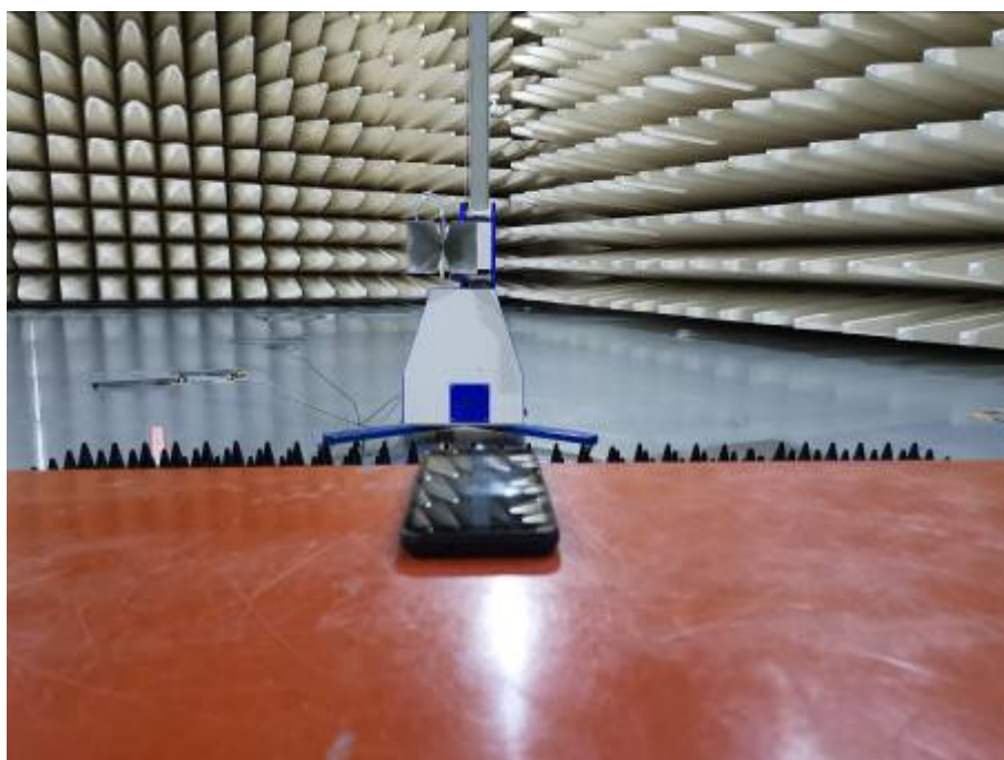
Radiated Emissions Test Setup (above1GHz)
