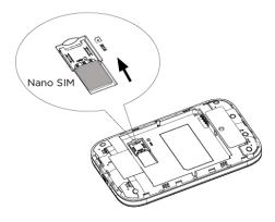
Insert the Nano SIM card. Install the battery and replace the back cover. When replacing the back cover, please ensure the back cover is aligned correctly.
