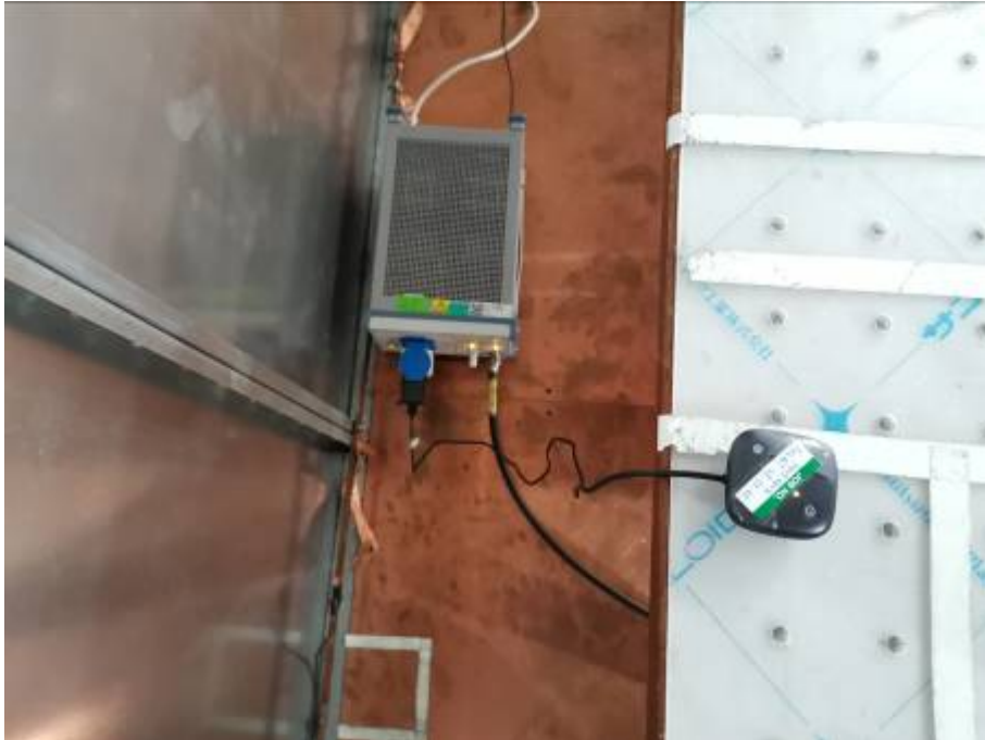
Conducted Emissions Test Setup
