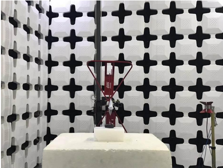
5. Radiated Emissions (Part 22/24/27) (30MHz-18GHz)
