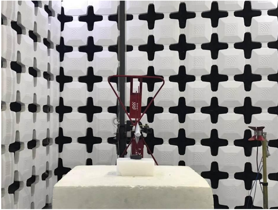
3. Radiated Emissions (Part 15C) (1-18GHz)
