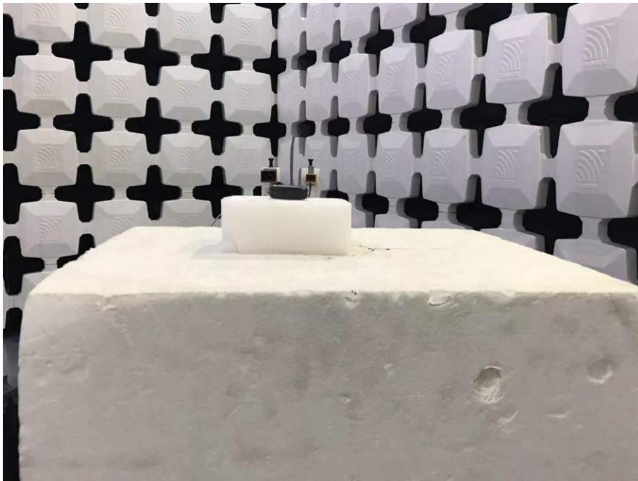
4. Radiated Emissions (Part 15C) (18-26.5GHz)
