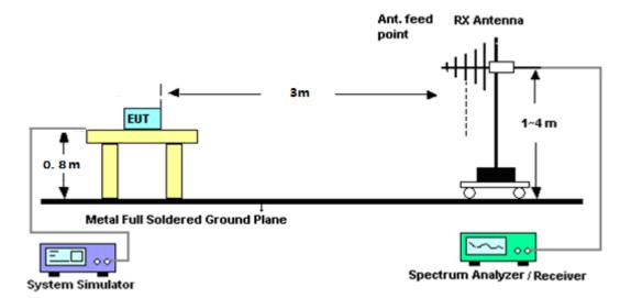
For radiated test from above 1GHz
