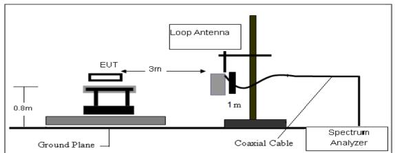
(B) Radiated Emission Test-Up Frequency 30MHz~1GHz
