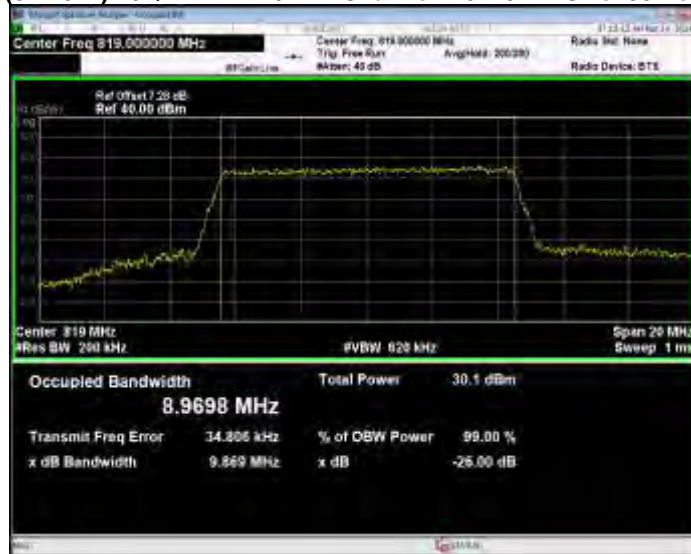
Band26(814-824) 16QAM BW=3MHz Channel=26705 RB Size=15 Position=#0
