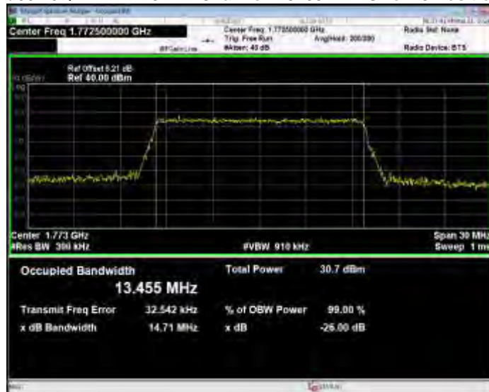
Band66 16QAM BW=20MHz Channel=132072 RB Size=100 Position=#0
