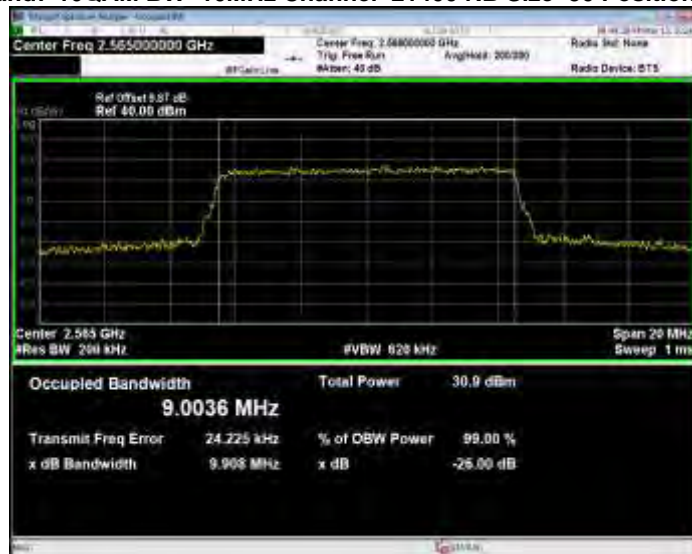
Band7 16QAM BW=10MHz Channel=21400 RB Size=50 Position=#0
