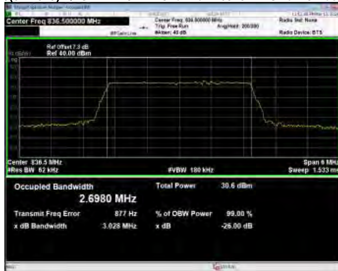
Band26(824-849) QPSK BW=3MHz Channel=27025 RB Size=15 Position=#0
