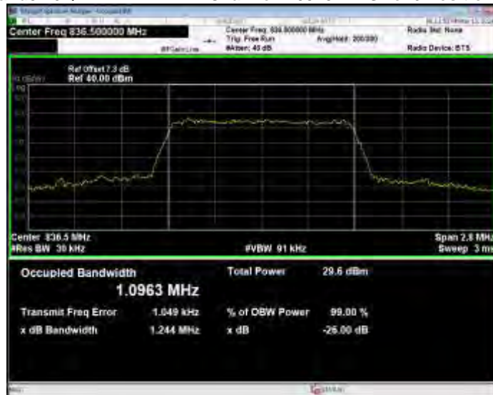
Band5 16QAM BW=1.4MHz Channel=20643 RB Size=6 Position=#0
