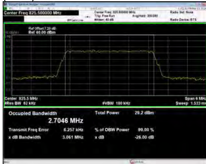
Band26(824-849) 16QAM BW=3MHz Channel=26805 RB Size=15 Position=#0
