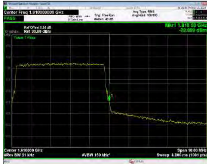
Band2 QPSK BW=5MHz Channel=19175 RB Size=25 Position=#0
