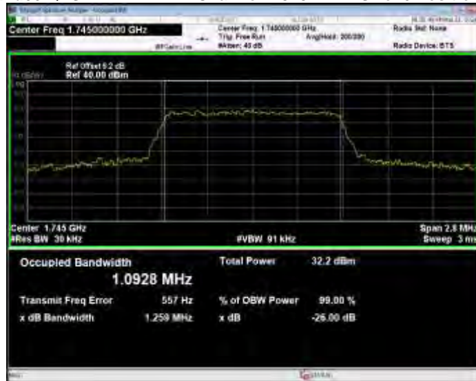
Band66 QPSK BW=1.4MHz Channel=132665 RB Size=6 Position=#0
