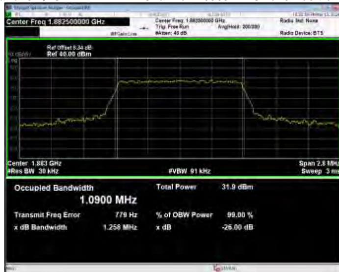
Band25 QPSK BW=1.4MHz Channel=26683 RB Size=6 Position=#0
