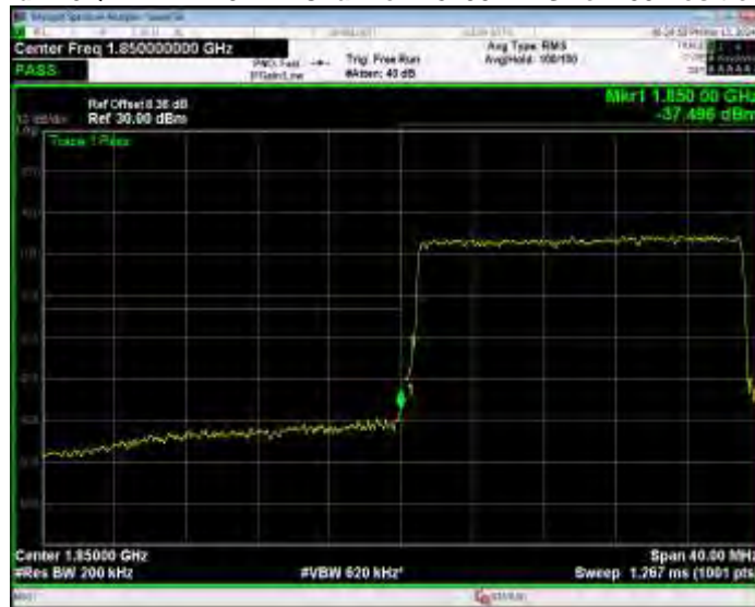
Band2 16QAM BW=20MHz Channel=19100 RB Size=1 Position=#0
