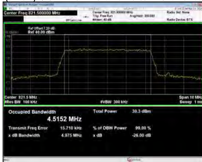
Band26(824-849) 16QAM BW=1.4MHz Channel=26797 RB Size=6 Position=#0
