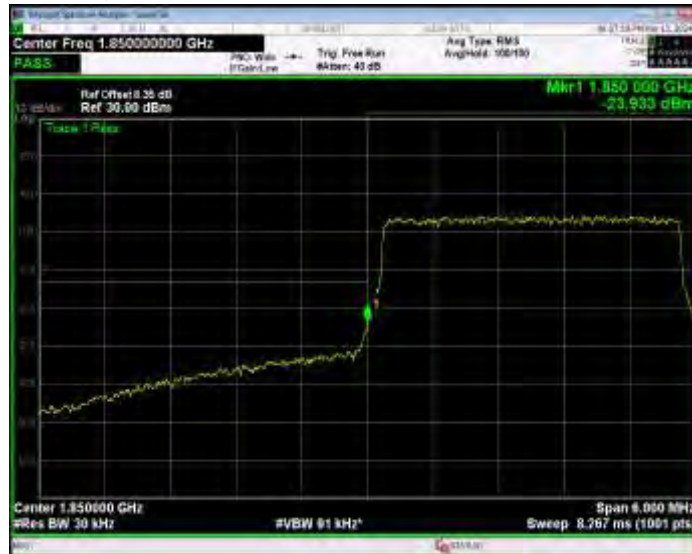
Band2 16QAM BW=3MHz Channel=18615 RB Size=15 Position=#0
