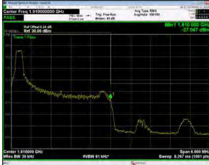
Band2 QPSK BW=3MHz Channel=19185 RB Size=15 Position=#0
