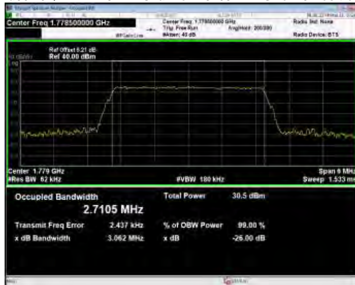
Band66 16QAM BW=5MHz Channel=131997 RB Size=25 Position=#0
