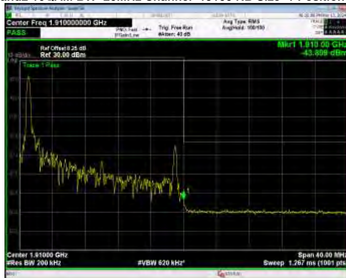
Band2 16QAM BW=20MHz Channel=19100 RB Size=1 Position=#0
