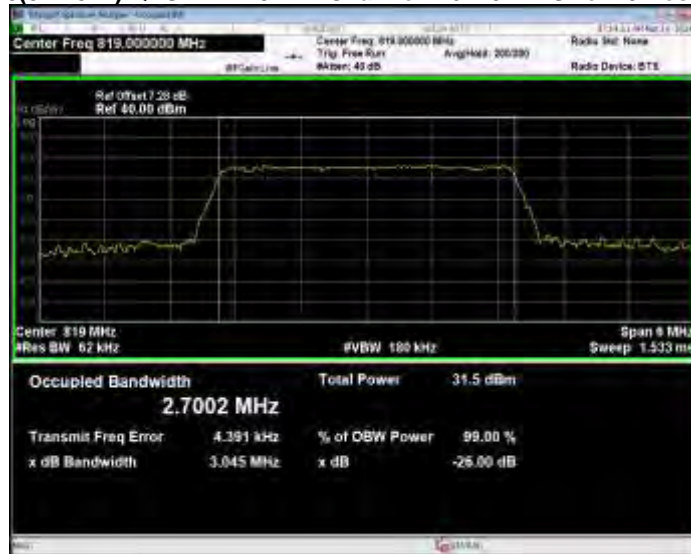
Band26(814-824) QPSK BW=3MHz Channel=26775 RB Size=15 Position=#0
