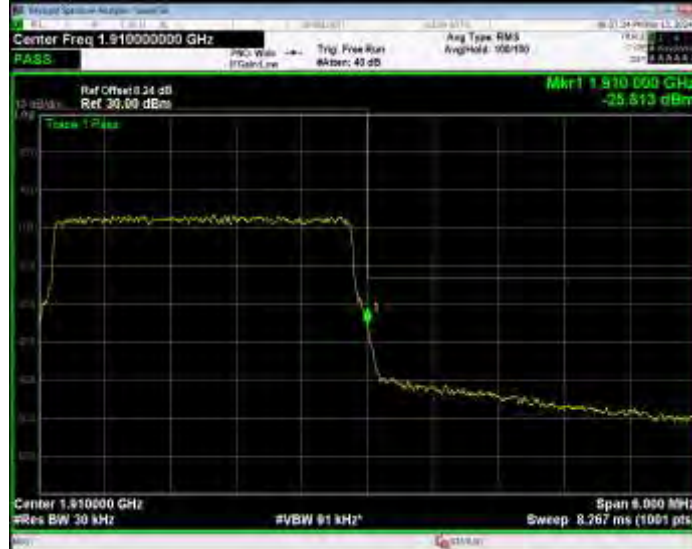
Band2 16QAM BW=5MHz Channel=18625 RB Size=1 Position=#0
