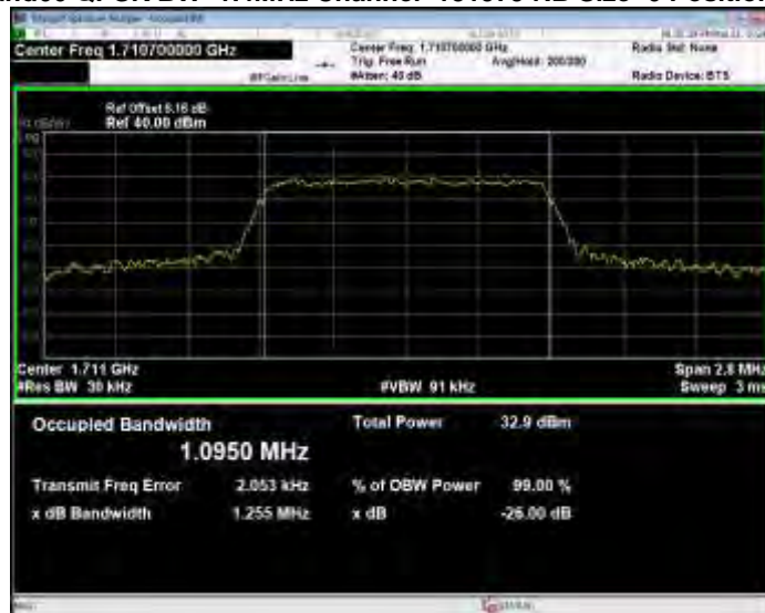
Band66 QPSK BW=1.4MHz Channel=131979 RB Size=6 Position=#0
