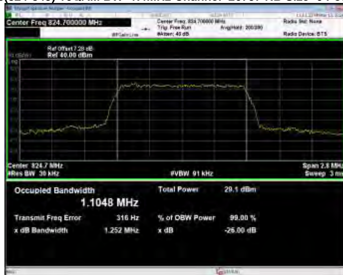
Band26(824-849) 16QAM BW=1.4MHz Channel=26797 RB Size=6 Position=#0
