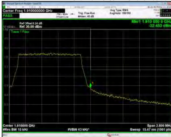
Band2 16QAM BW=10MHz Channel=18650 RB Size=1 Position=#0
