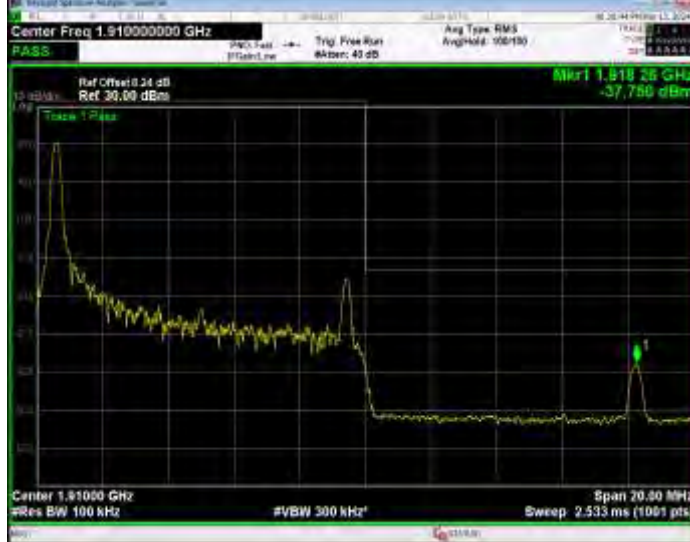
Band2 QPSK BW=10MHz Channel=19150 RB Size=50 Position=#0
