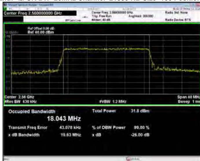
Band7 QPSK BW=20MHz Channel=21350 RB Size=100 Position=#0
