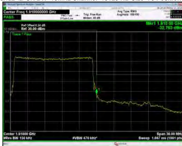
Band2 QPSK BW=15MHz Channel=19125 RB Size=75 Position=#0
