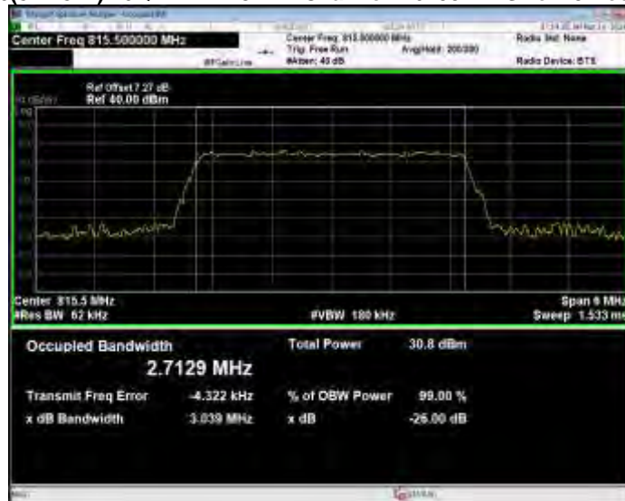
Band26(814-824) 16QAM BW=3MHz Channel=26740 RB Size=15 Position=#0
