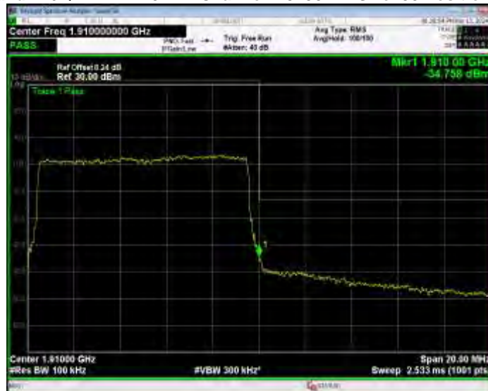
Band2 16QAM BW=15MHz Channel=18675 RB Size=1 Position=#0
