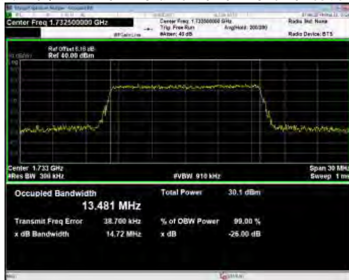
Band4 16QAM BW=15MHz Channel=20325 RB Size=75 Position=#0
