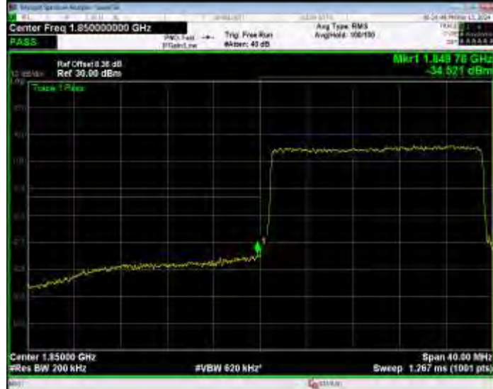
Band2 QPSK BW=20MHz Channel=19100 RB Size=1 Position=#0
