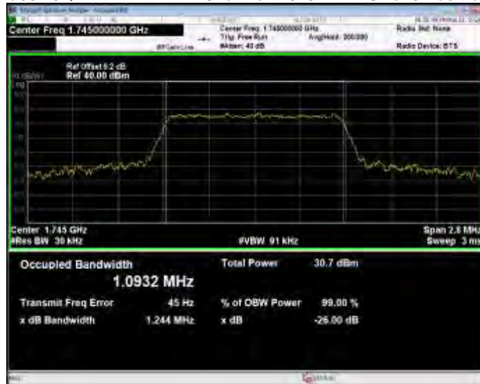
Band66 16QAM BW=1.4MHz Channel=132665 RB Size=6 Position=#0
