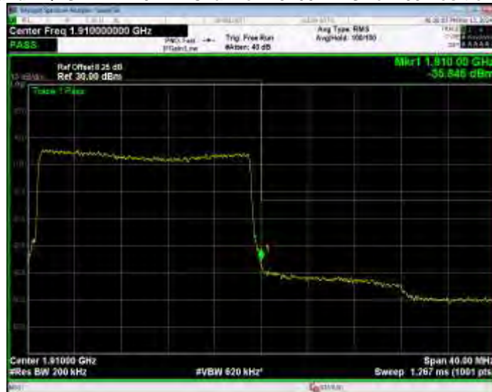
Band2 QPSK BW=3MHz Channel=18615 RB Size=1 Position=#0
