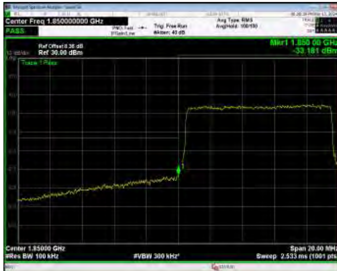
Band2 16QAM BW=10MHz Channel=18650 RB Size=50 Position=#0
