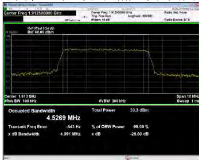
Band25 16QAM BW=5MHz Channel=26665 RB Size=25 Position=#0
