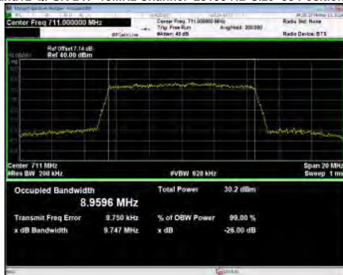
Band12 QPSK BW=10MHz Channel=23130 RB Size=50 Position=#0
