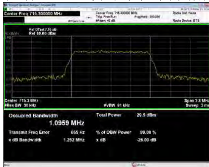
Band12 16QAM BW=1.4MHz Channel=23173 RB Size=6 Position=#0
