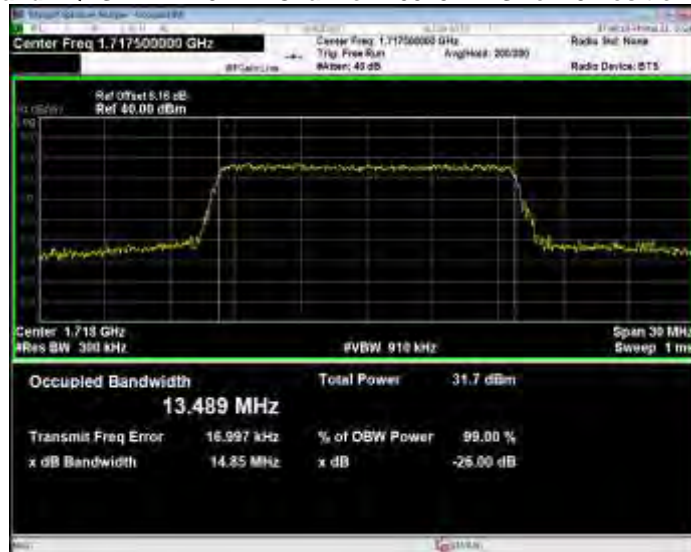
Band4 QPSK BW=15MHz Channel=20175 RB Size=75 Position=#0
