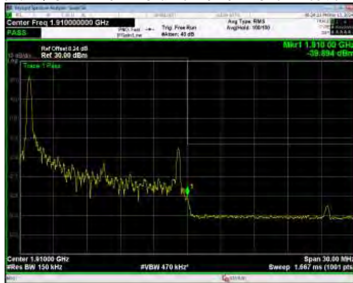
Band2 QPSK BW=15MHz Channel=19125 RB Size=75 Position=#0
