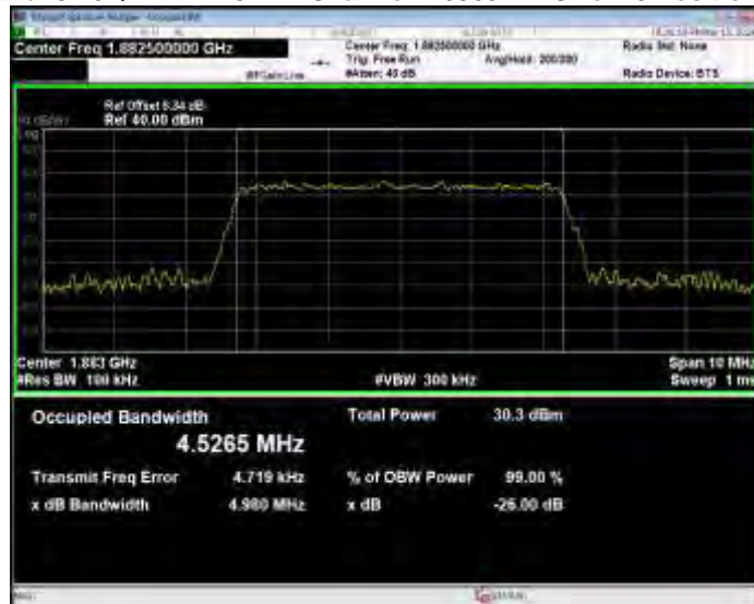
Band25 16QAM BW=5MHz Channel=26665 RB Size=25 Position=#0
