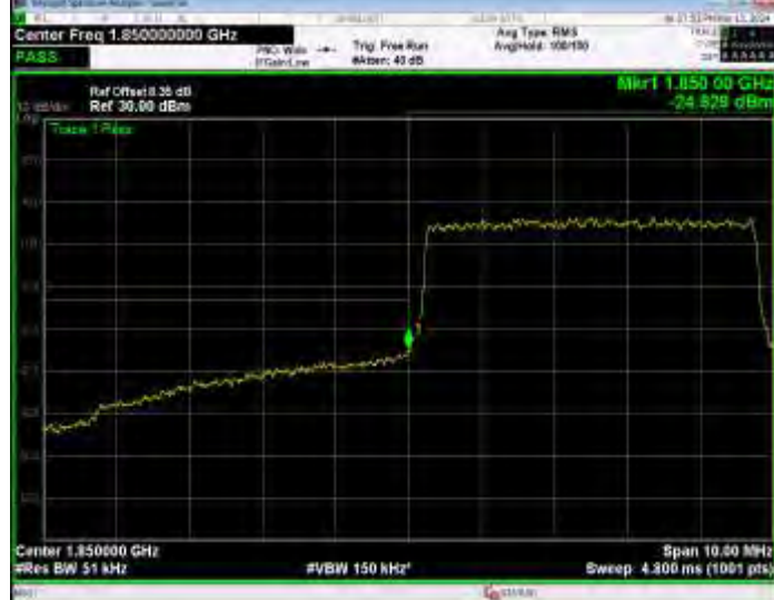
Band2 QPSK BW=5MHz Channel=19175 RB Size=1 Position=#0
