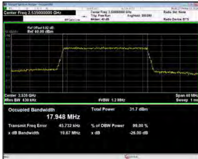
Band7 QPSK BW=20MHz Channel=21350 RB Size=100 Position=#0
