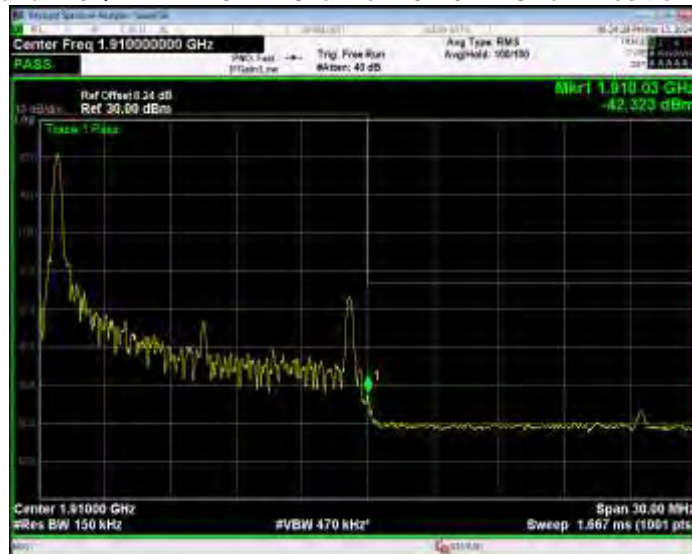
Band2 16QAM BW=15MHz Channel=19125 RB Size=75 Position=#0
