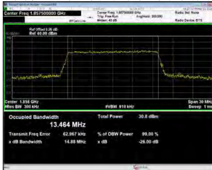
Band25 16QAM BW=15MHz Channel=26365 RB Size=75 Position=#0
