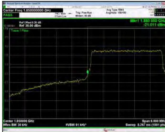
Band2 QPSK BW=3MHz Channel=18615 RB Size=15 Position=#0
