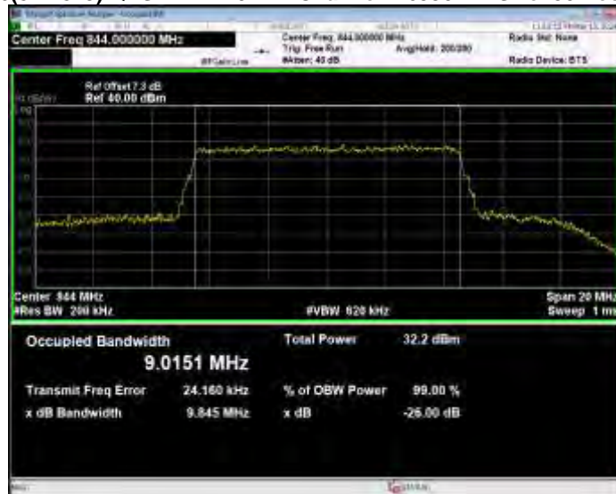
Band26(824-849) QPSK BW=15MHz Channel=26865 RB Size=75 Position=#0
