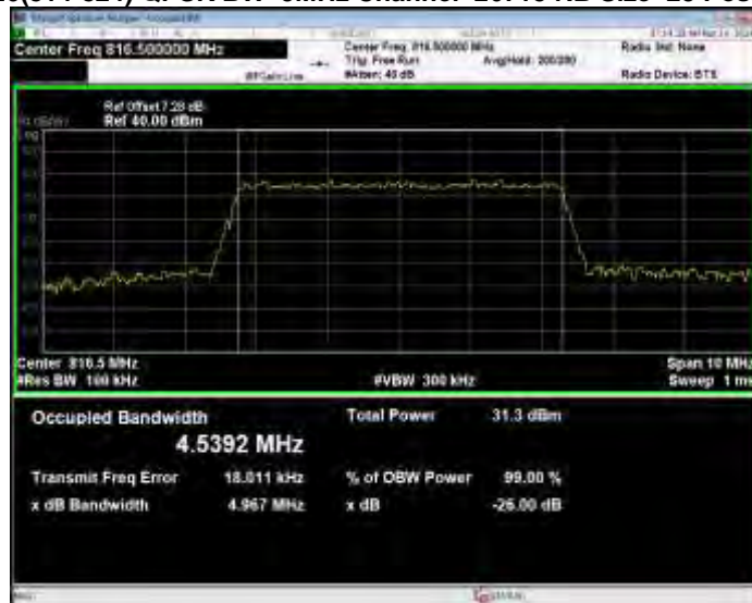
Band26(814-824) QPSK BW=5MHz Channel=26715 RB Size=25 Position=#0
