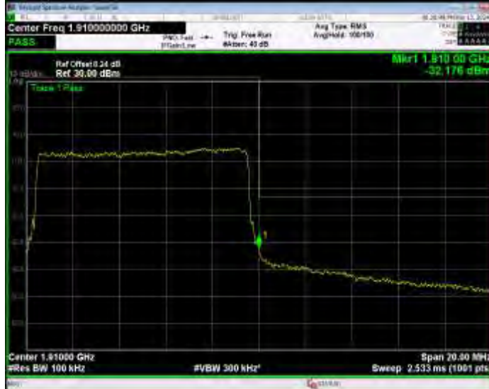
Band2 QPSK BW=15MHz Channel=18675 RB Size=1 Position=#0
