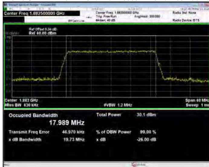
Band25 16QAM BW=20MHz Channel=26590 RB Size=100 Position=#0
