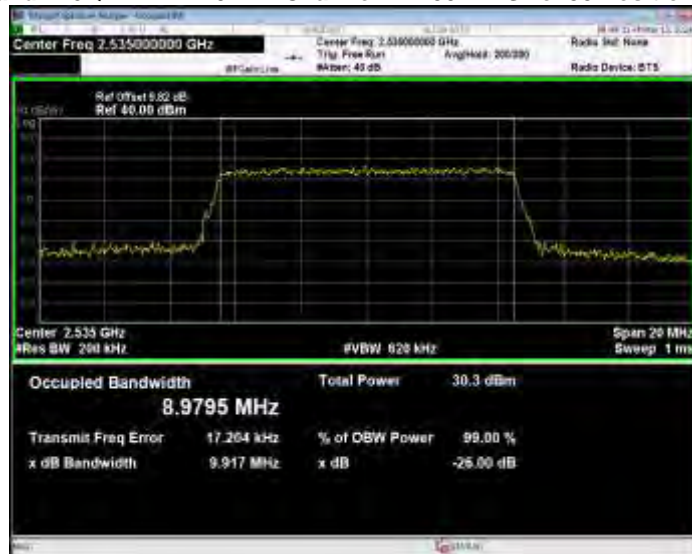
Band7 16QAM BW=10MHz Channel=21400 RB Size=50 Position=#0
