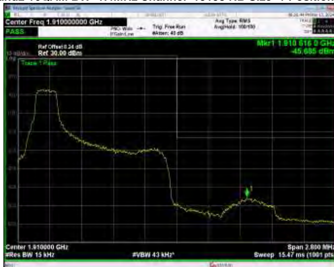
Band2 16QAM BW=1.4MHz Channel=19193 RB Size=1 Position=#0
