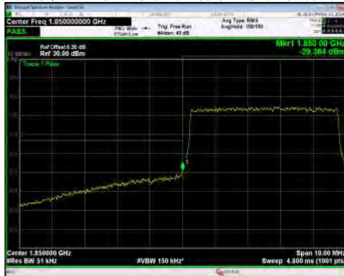
Band2 16QAM BW=5MHz Channel=19175 RB Size=1 Position=#0
