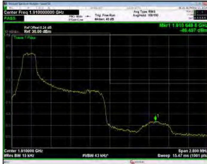
Band2 QPSK BW=1.4MHz Channel=19193 RB Size=1 Position=#0
