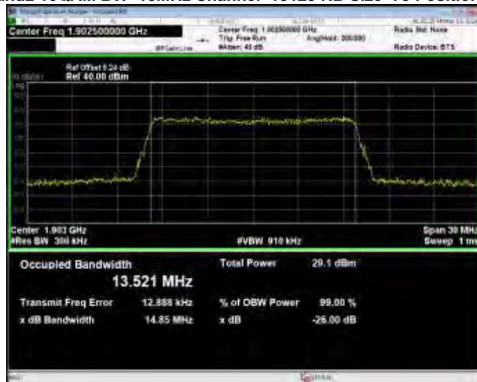
Band2 16QAM BW=15MHz Channel=19125 RB Size=75 Position=#0
