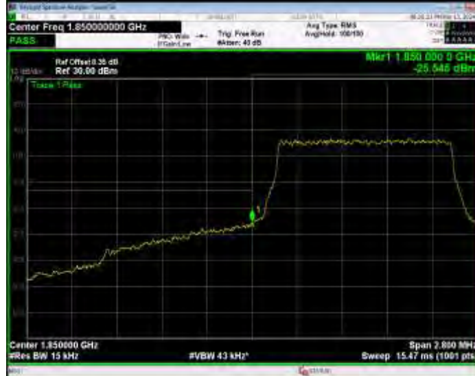
Band2 QPSK BW=1.4MHz Channel=19193 RB Size=1 Position=#0
