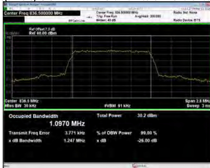
Band26(824-849) QPSK BW=1.4MHz Channel=27033 RB Size=6 Position=#0
