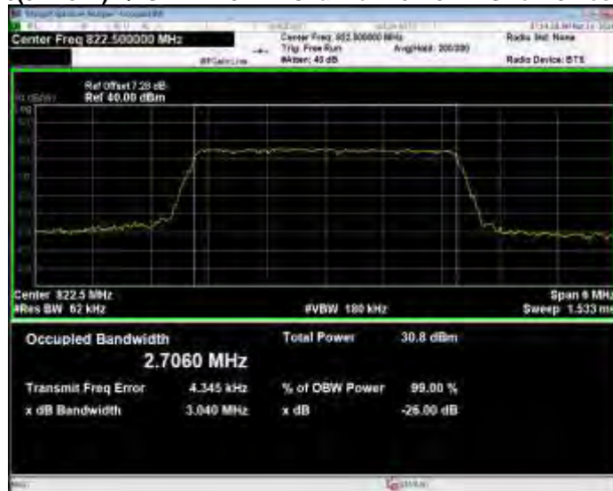
Band26(814-824) QPSK BW=5MHz Channel=26715 RB Size=25 Position=#0
