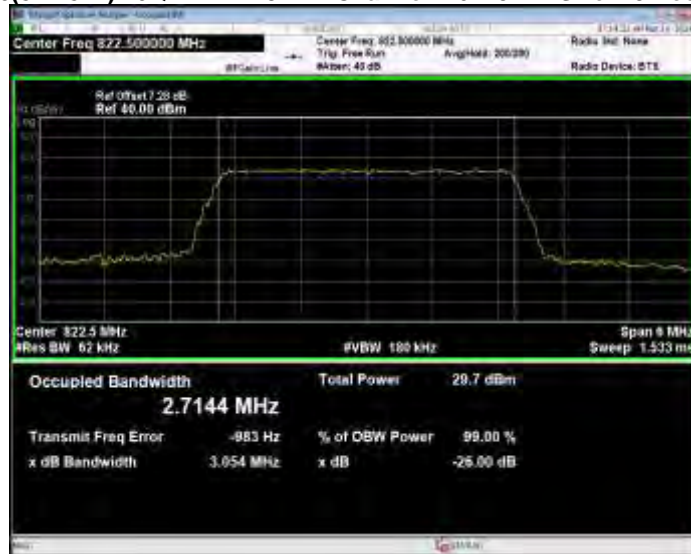
Band26(814-824) 16QAM BW=5MHz Channel=26715 RB Size=25 Position=#0
