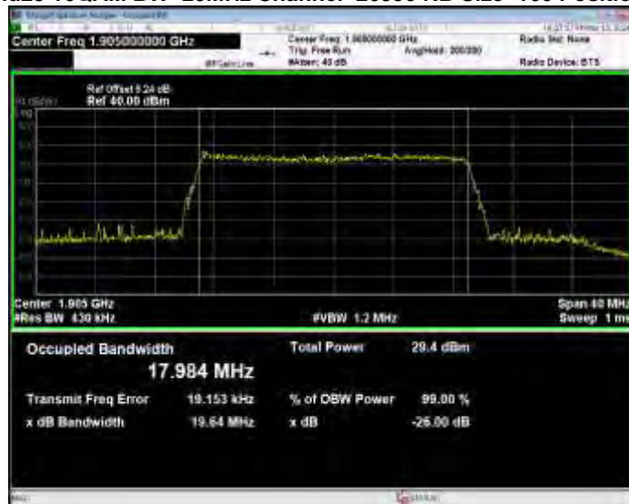
Band25 16QAM BW=20MHz Channel=26590 RB Size=100 Position=#0
