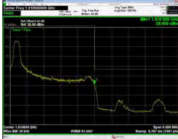
Band2 16QAM BW=3MHz Channel=19185 RB Size=15 Position=#0
