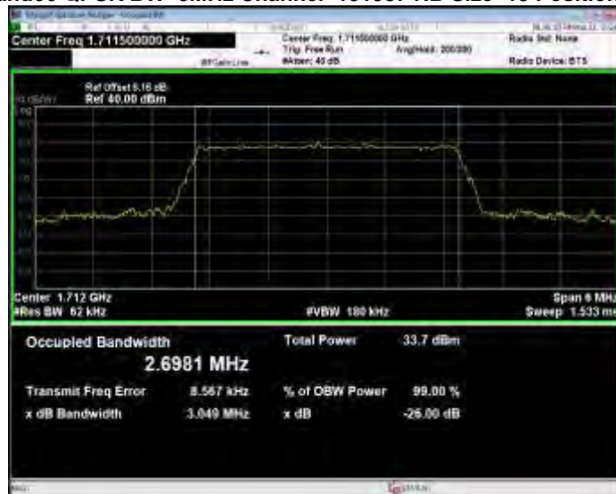
Band66 QPSK BW=3MHz Channel=131987 RB Size=15 Position=#0
