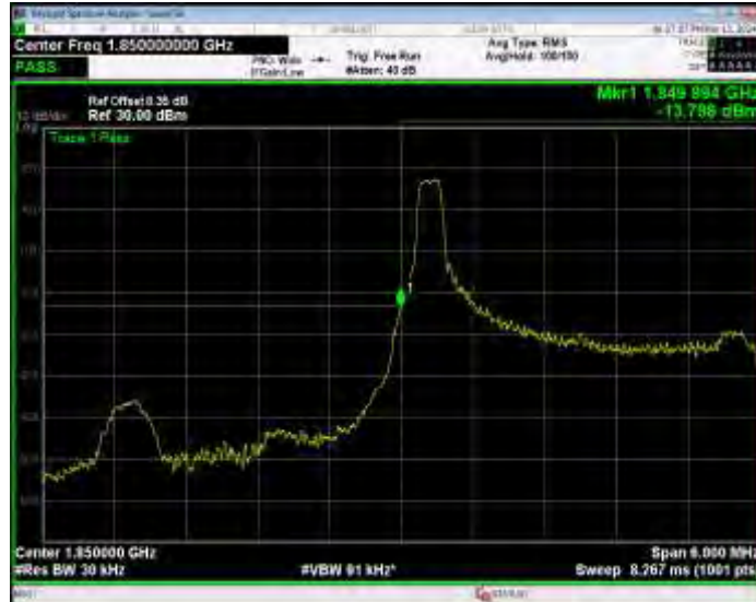
Band2 QPSK BW=3MHz Channel=18615 RB Size=15 Position=#0
