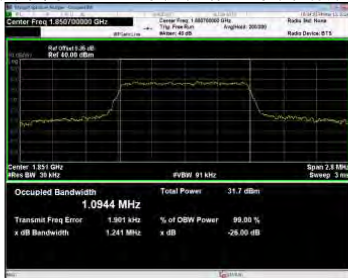
Band25 QPSK BW=1.4MHz Channel=26365 RB Size=6 Position=#0
