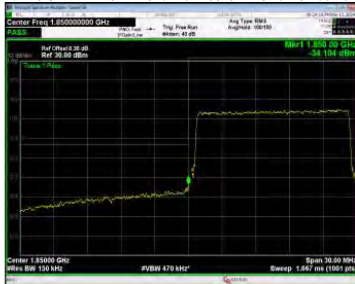
Band2 16QAM BW=15MHz Channel=19125 RB Size=1 Position=#0
