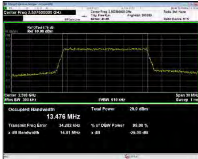
Band7 16QAM BW=15MHz Channel=21100 RB Size=75 Position=#0
