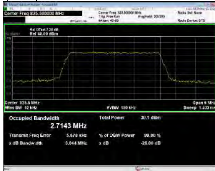
Band26(824-849) QPSK BW=3MHz Channel=26805 RB Size=15 Position=#0
