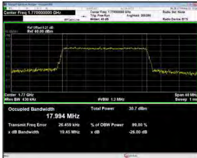
Band66 16QAM BW=3MHz Channel=131987 RB Size=15 Position=#0
