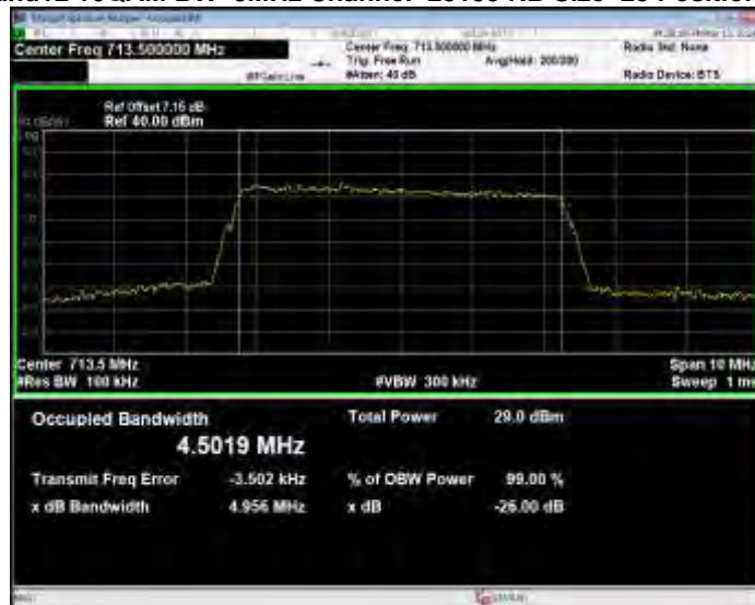
Band12 16QAM BW=5MHz Channel=23155 RB Size=25 Position=#0
