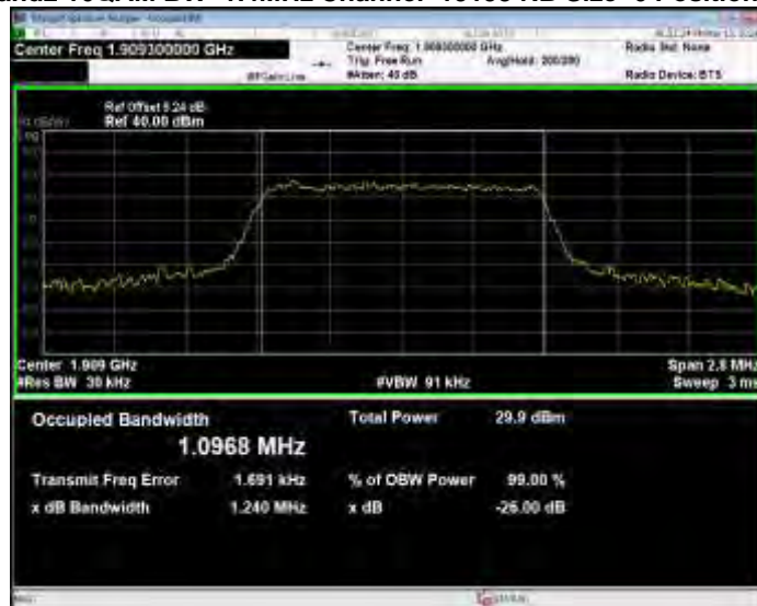
Band2 16QAM BW=1.4MHz Channel=19193 RB Size=6 Position=#0
