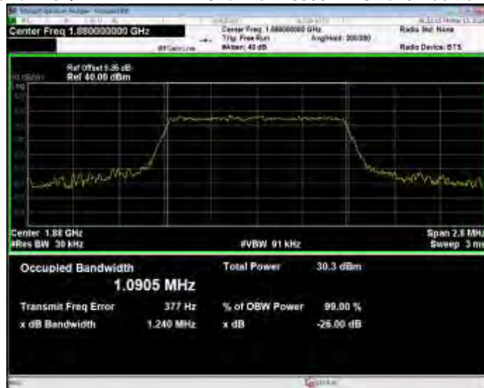
Band2 16QAM BW=1.4MHz Channel=19193 RB Size=6 Position=#0
