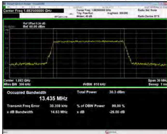
Band25 16QAM BW=15MHz Channel=26615 RB Size=75 Position=#0
