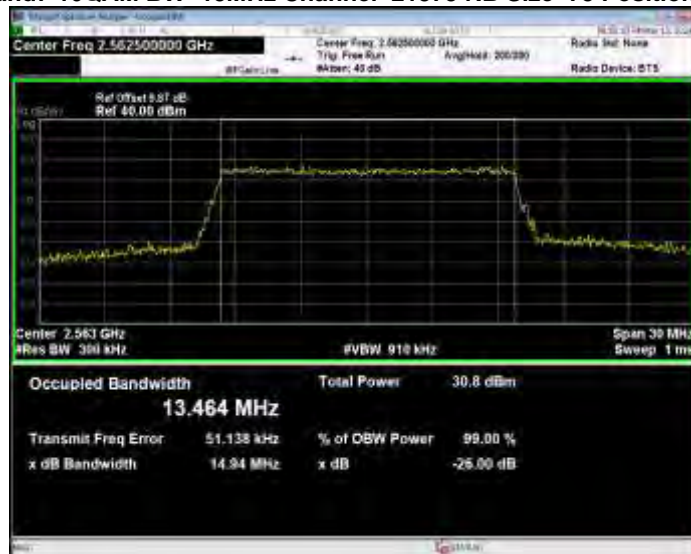
Band7 16QAM BW=15MHz Channel=21375 RB Size=75 Position=#0
