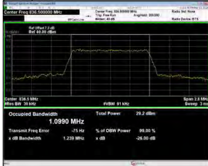
Band26(824-849) 16QAM BW=1.4MHz Channel=27033 RB Size=6 Position=#0
