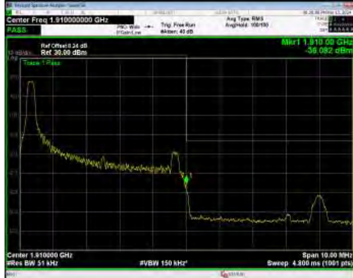
Band2 QPSK BW=5MHz Channel=19175 RB Size=25 Position=#0
