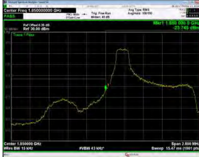
Band2 QPSK BW=1.4MHz Channel=18607 RB Size=6 Position=#0
