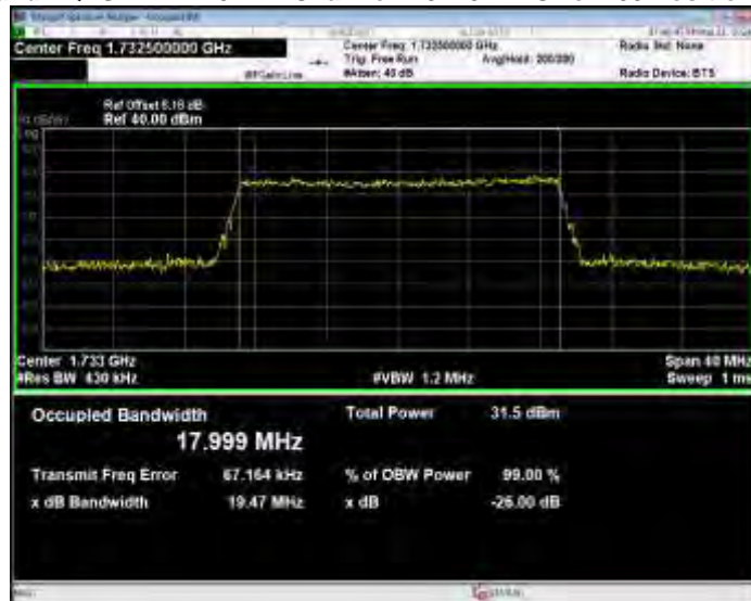
Band4 QPSK BW=20MHz Channel=20300 RB Size=100 Position=#0
