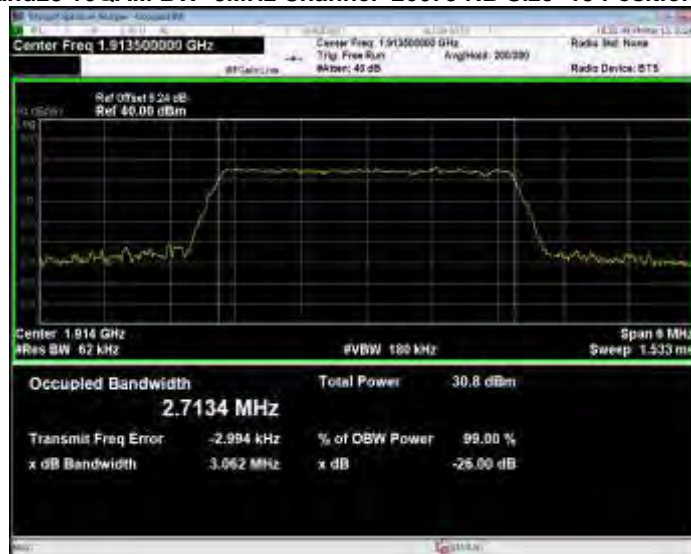
Band25 16QAM BW=3MHz Channel=26675 RB Size=15 Position=#0
