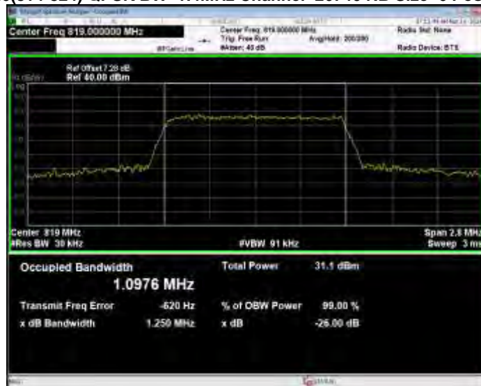
Band26(814-824) QPSK BW=1.4MHz Channel=26740 RB Size=6 Position=#0
