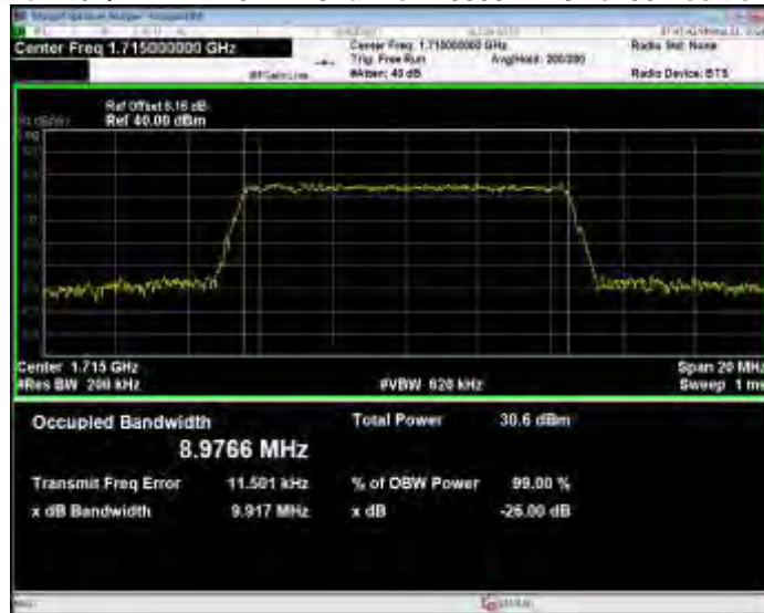
Band4 16QAM BW=10MHz Channel=20175 RB Size=50 Position=#0
