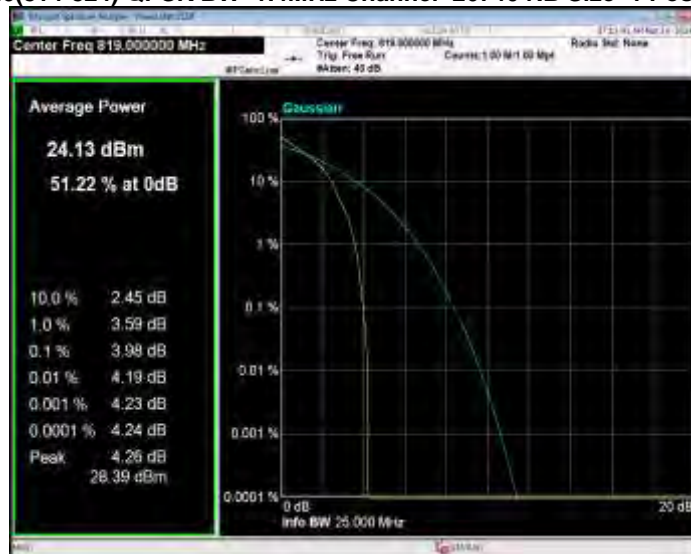
Band26(814-824) QPSK BW=1.4MHz Channel=26740 RB Size=1 Position=#0
