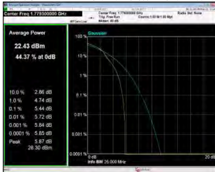
Band66 16QAM BW=10MHz Channel=132022 RB Size=1 Position=#0
