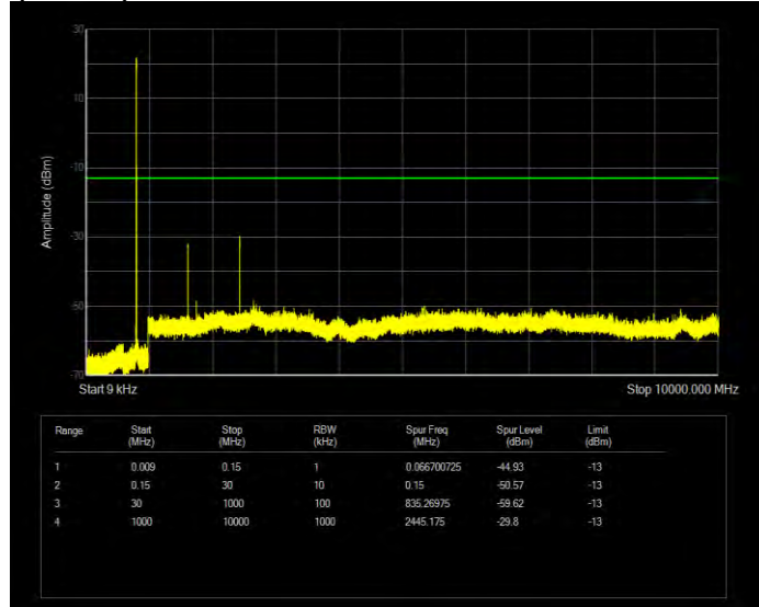
Band26(814-824) QPSK BW=1.4MHz Channel=26740 RB Size=6 Position=#0
