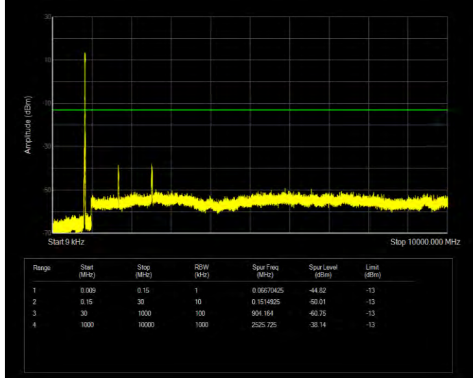
Band26(824-849) 16QAM BW=15MHz Channel=26865 RB Size=75 Position=#0
