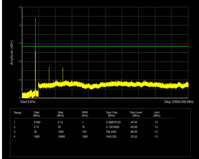
Band26(814-824) QPSK BW=5MHz Channel=26715 RB Size=25 Position=#0
