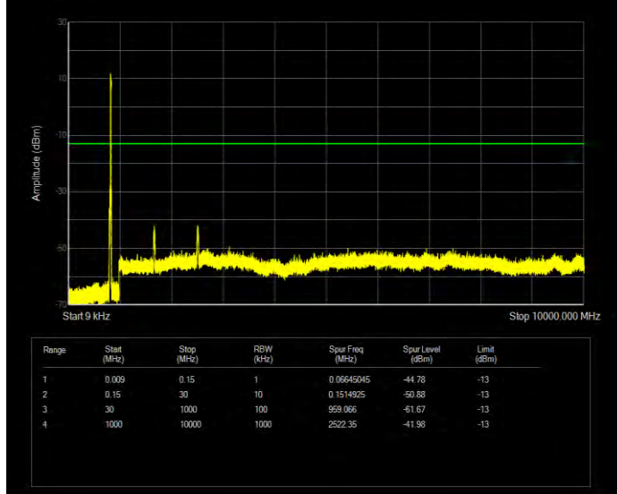
Band26(824-849) 16QAM BW=3MHz Channel=26805 RB Size=15 Position=#0
