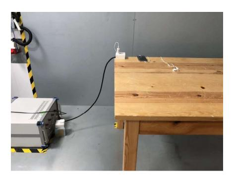
Set-up for Radiated Emission (RE), Below 1GHz
