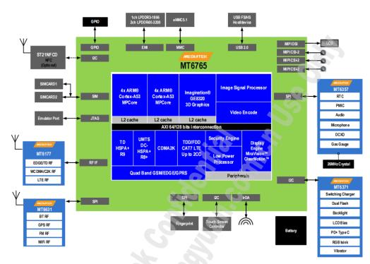
Figure 1-1. High-level MT6765X functional block diagram
