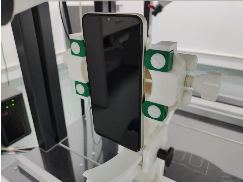
Body Top side (separation distance is 10mm)
