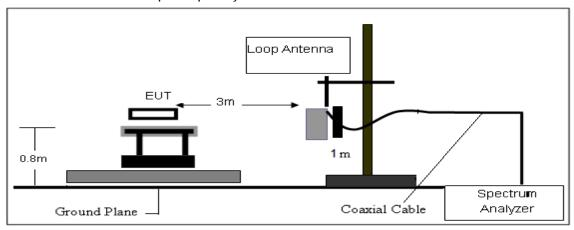
(B) Radiated Emission Test-Up Frequency 30MHz~1GHz
