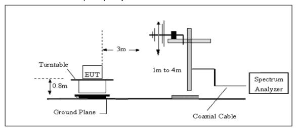
(C) Radiated Emission Test-Up Frequency Above 1GHz
