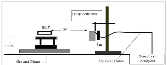
(B) Radiated Emission Test-Up Frequency 30MHz~1GHz
