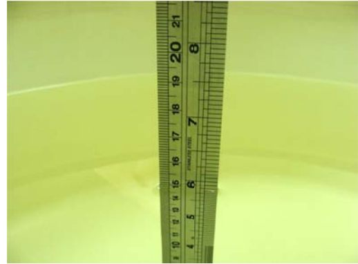
Fig 6.2 Photo of Liquid Height for Body SAR
