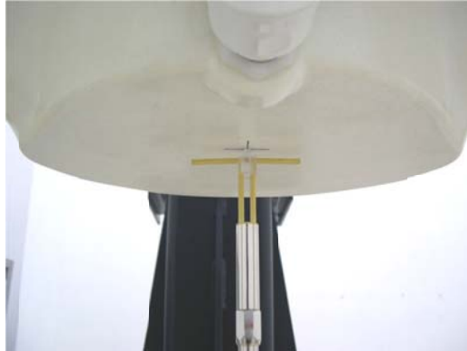
Fig 7.2 Photo of Dipole Setup
