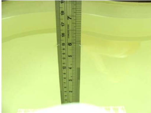
Fig 6.1 Photo of Liquid Height for Head SAR
