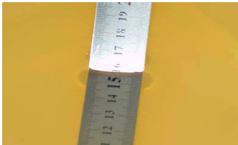
Fig47: Liquid depth for SAR Measurement
