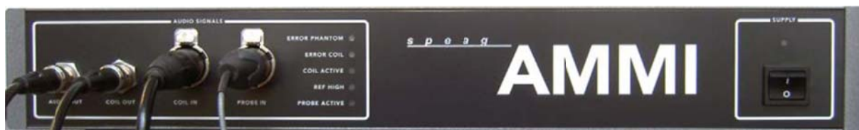
Fig. 5.3 AMMI front panel
