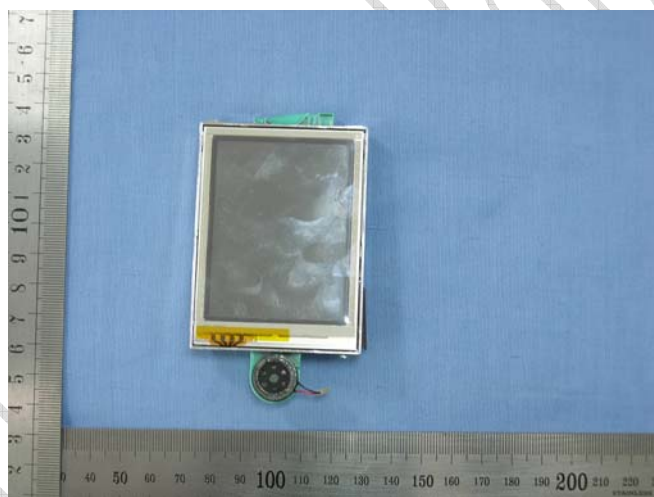
Picture 6 Front view of the internal structure (LCD)
