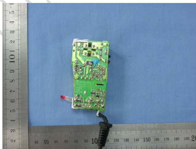
Picture 13 back view of adaptor internal structure
