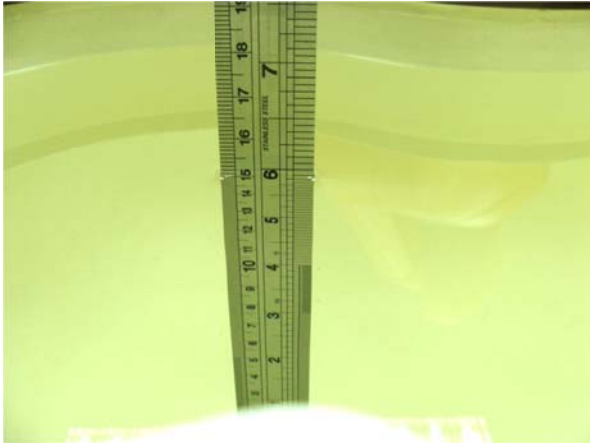
Fig 6.1 Photo of Liquid Height for Head SAR
