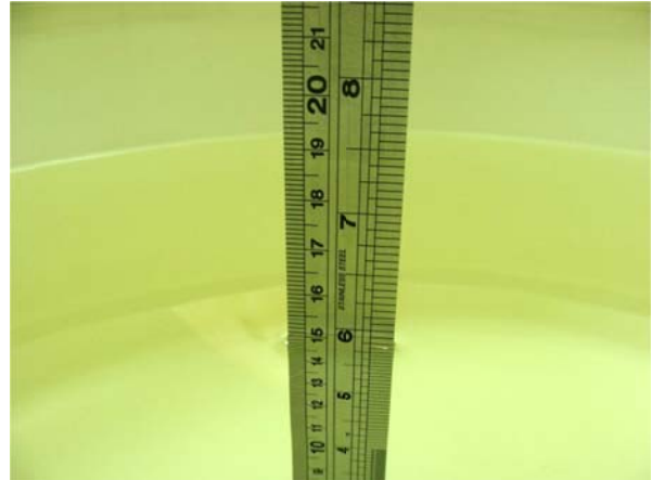
Fig 6.2 Photo of Liquid Height for Body SAR
