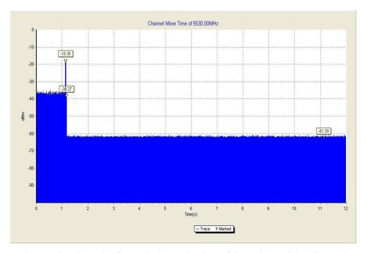
The channel move time is as the figure. It shows the time of the radar and the client pulses. The figure shows that the client stops transmission within 10 seconds, and no transmissions occur after 10 seconds later of the radar burst signal.
