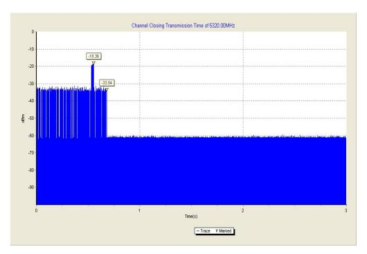
The closing transmission time is as the figure, and the result is 101ms.
