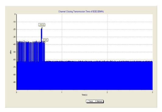
The closing transmission time is as the figure, and the result is 200ms.
