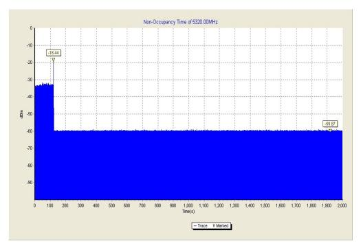
The figure above shows that the client does not transmit any emission within 1800 seconds after getting the order of "stop transmits" from the DFS master (access point).
