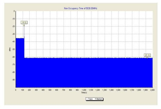
The figure above shows that the client does not transmit any emission within 1800 seconds after getting the order of "stop transmits" from the DFS master (access point).
