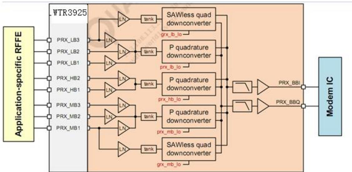
The serial signal mobile received go to RF Connector, and then transmit to transceiver WTR3925 via the selected band in RF switcher&SAW filter.IQ signals input to Transceiver for demodulation and de-code, then go to Base band.
