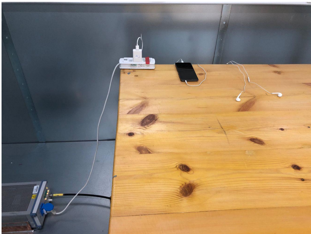
16. Conducted Emission (Part 15B Charging mode-FM)
