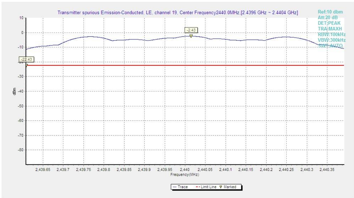
Fig.12 Conducted Spurious Emission (Ch19, Center Frequency)
