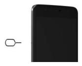
1. Insert the ejection pin into the hole to open the SIM card tray.
