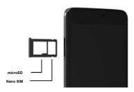
2. Gently pull out the SIM card tray gently. Place the Nano SIM card in card slot 1. If you have a microSD card (sold separately) place it in card slot 2.
