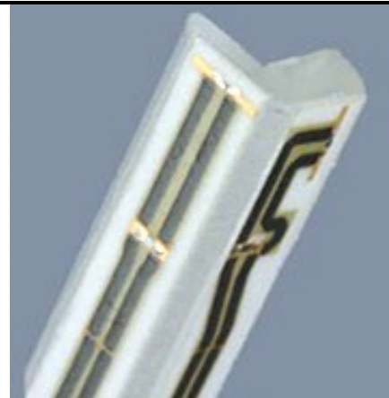
Fig 5.2 Photo of E-field Probe
