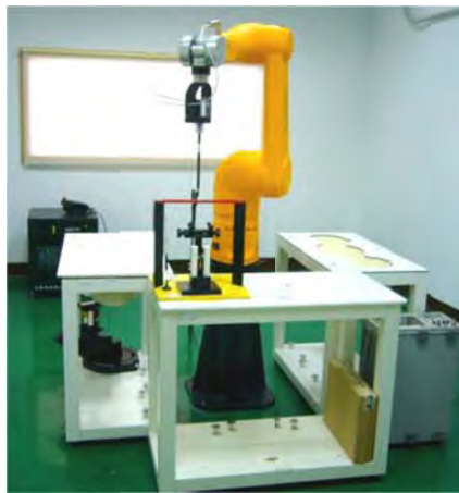
Fig 5.7 Photo of DASY5
