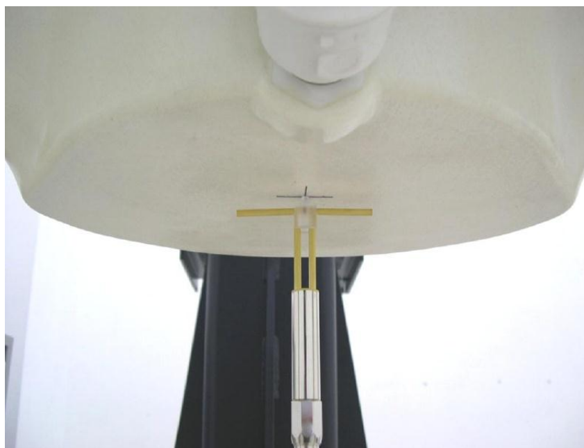
Picture 8.2 Photo of Dipole Setup
