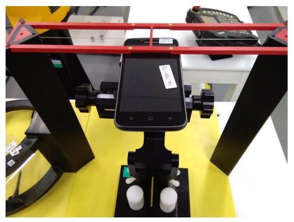
Picture 2: EUT Positioning for RF/T-coil
