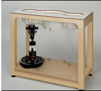
Picture C.8: SAM Twin Phantom
