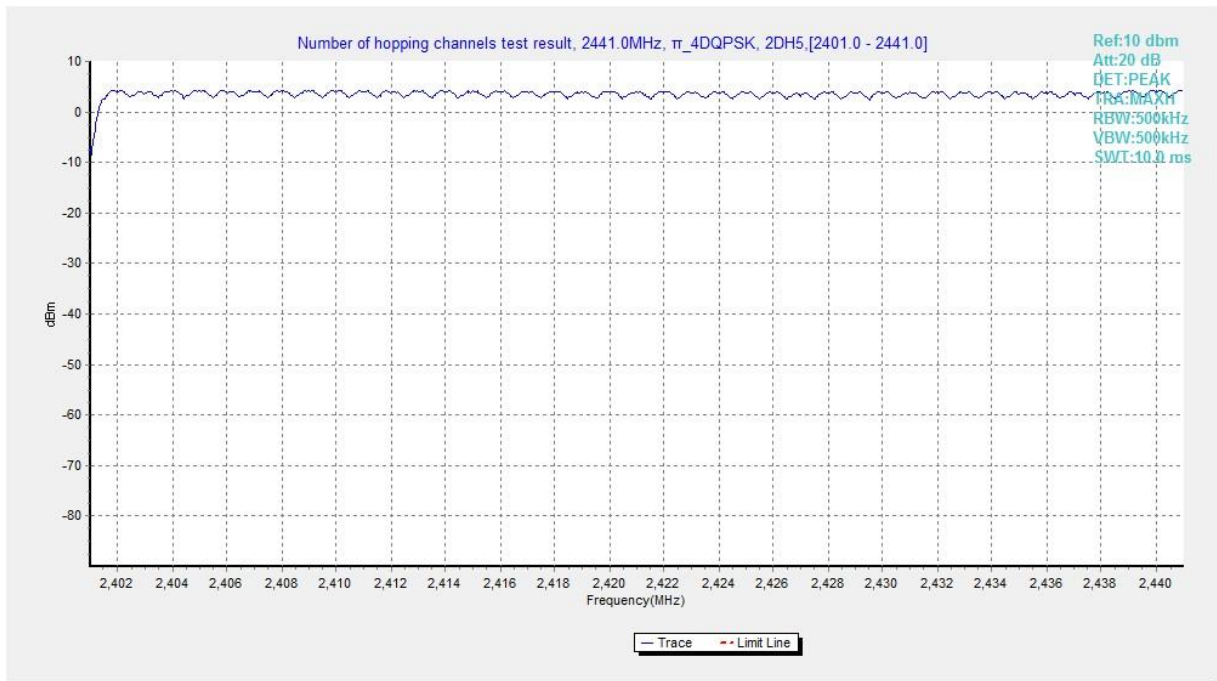
Fig. 77 Hopping channel ch0~39 ( \pi/4 DQPSK, Ch39)
