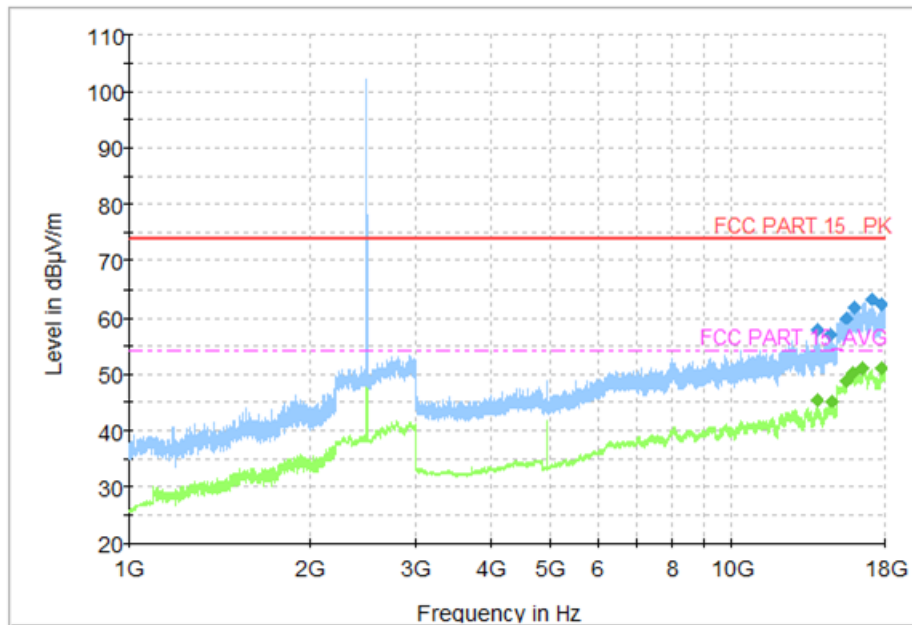
Fig. 44 Radiated Spurious Emission (GFSK, Ch78, 1 GHz ~18 GHz)
