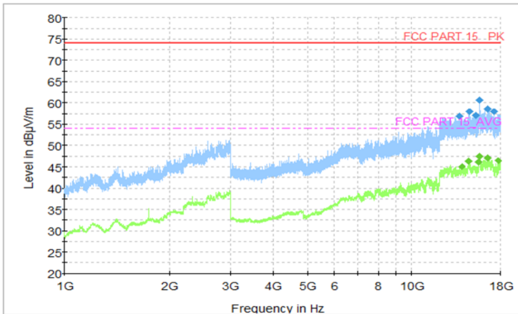
Figure A.10 Radiated Emission from 1GHz to 18GHz
