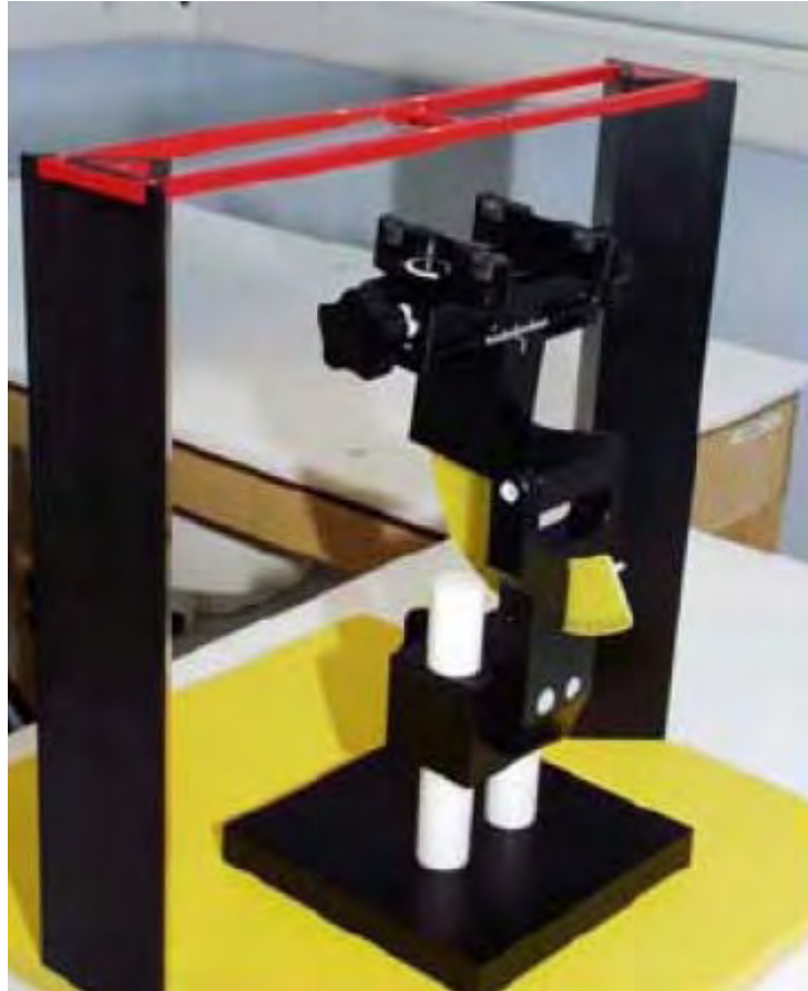
Figure 7 T-coil Phantom & Device Holder
