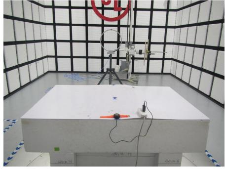
POWERLINE CONDUCTED EMISSIONS MEASUREMENT SETUP
